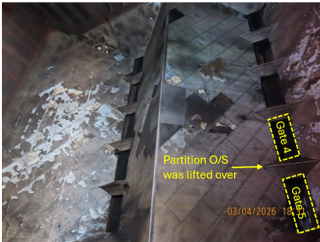
Bottom of cargo hold 4 (left) and gate 4 (right) after O/S was removed
