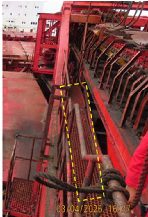
Catwalk (highlighted in yellow) fitted on boom conveyor (starboard side)
