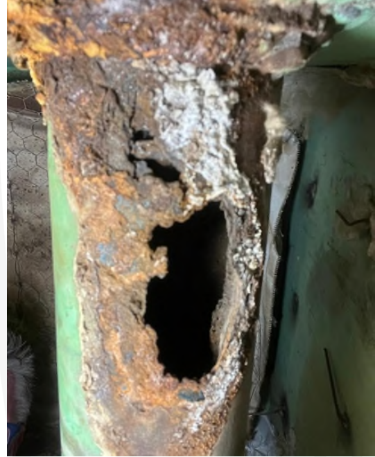
Flanged connection for level transmitter near corroded M4 ventilation pipe (to atmosphere)
