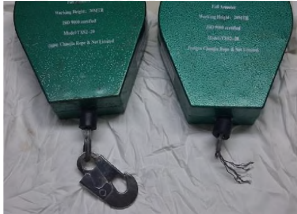
Undamaged sample with the failed fall arrestor
