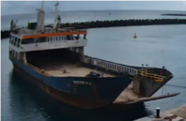
Port and Starboard side of Master RU with no prominent Load Line or draught marks
