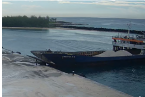
Port and Starboard side of Master RU with no prominent Load Line or draught marks
