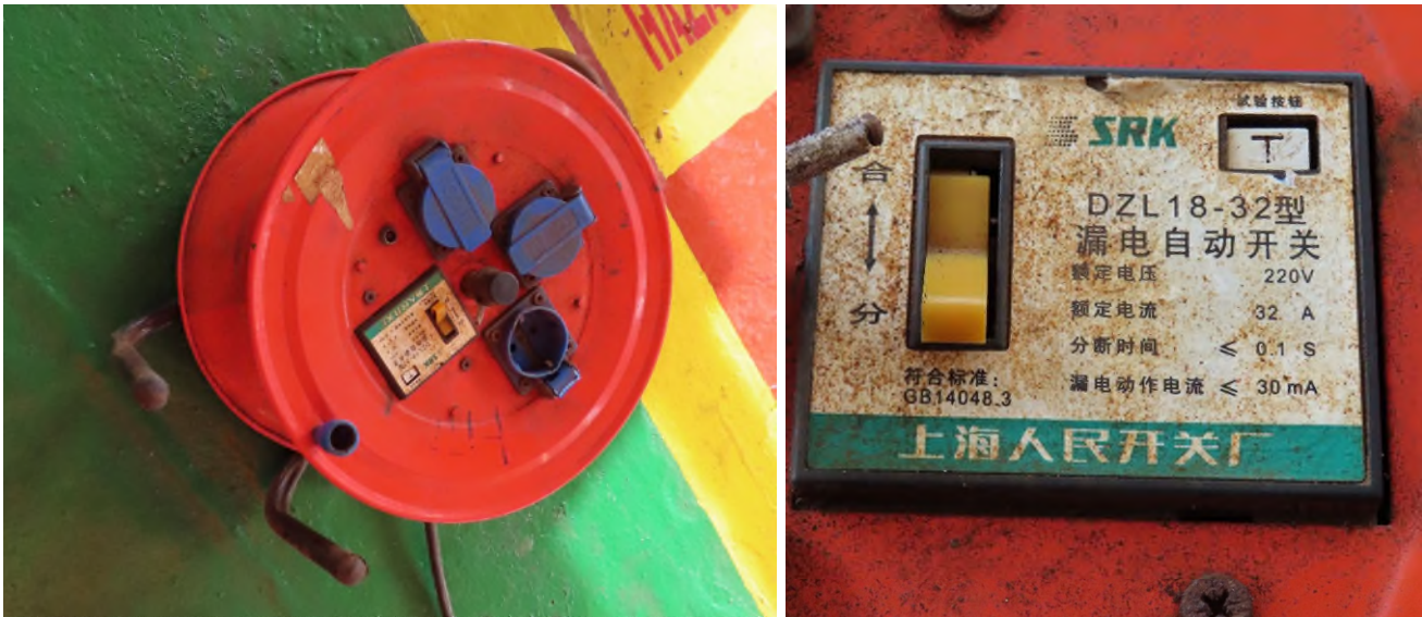
Extension cable reel. Detail of residual current device
