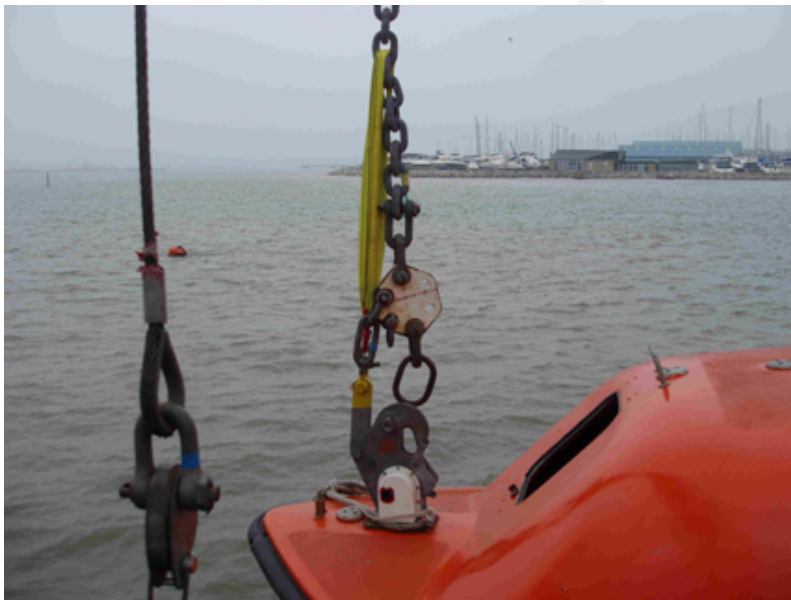
Figure 2 - FPD taking load during exercise, simulating premature release of on-load hook. Note that the boat is not waterborne but suspended just above the water - a safety precaution for avoiding injury to personnel or damage to structures during the exercise.
