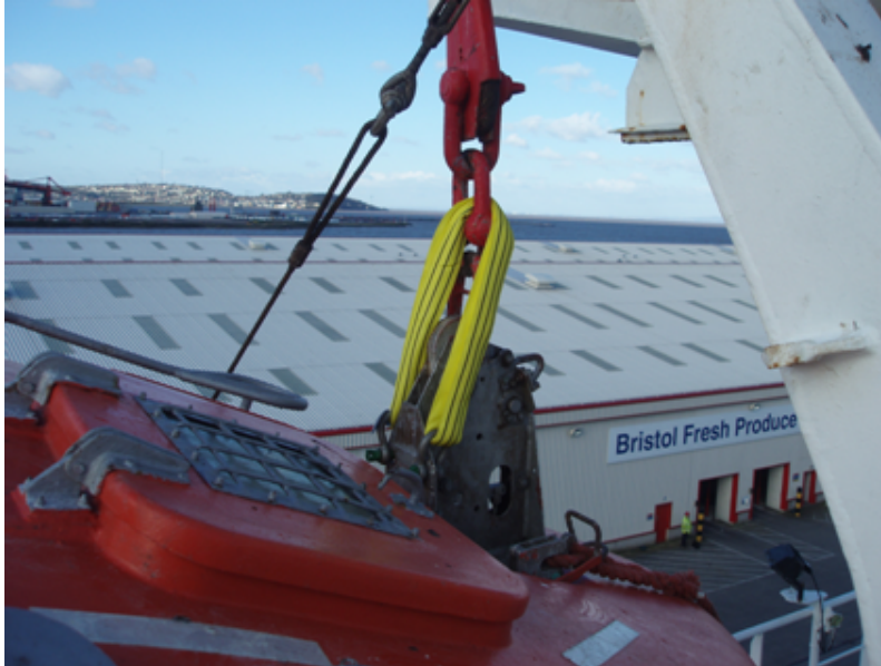
Figure 1 - Continuous sling in place over-riding on-load release
