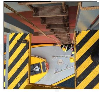
6.9. When a combination arrangement in use, the lower platform should be a minimum of 5 metres above sea level:
