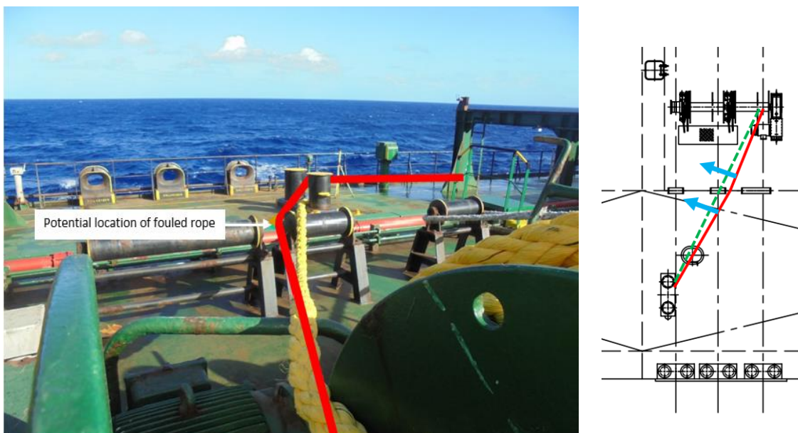
Figure 5. Illustration of fouled mooring line and directional force when released
