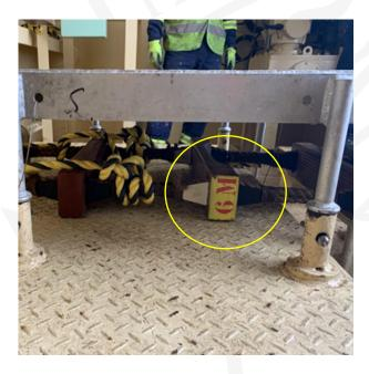
5.12. The side ropes of the pilot ladder should consist of two uncovered ropes not less than 18 millimetres in diameter on each side and should be continuous, with no joints and have a breaking strength of at least 24 kilonewtons (kN)<sup>5</sup> per rope:
