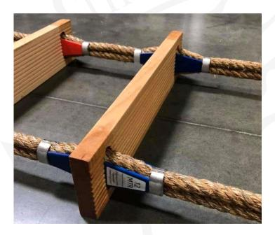
5.16. All pilot ladders used for pilot transfer shall be clearly identified with tags or other permanent marking so to enable identification of each appliance for the purposes of survey, inspection and record keeping:
