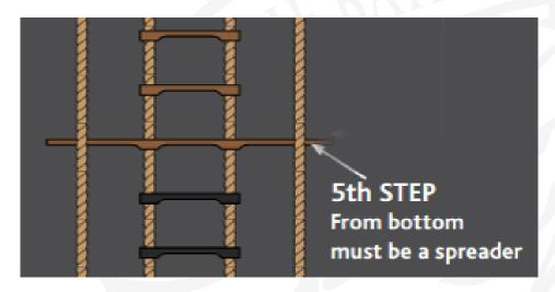
5.10. The lowest spreader step should be the fifth step from the bottom of the ladder and the interval between two spreader steps should not exceed nine steps.
