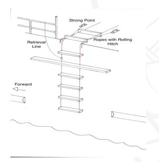
Note the cut in the rubbing band such that each step rests firmly against the ship's side and to allow a safe approach for pilot boat without the gunwale becoming trapped underneath the belting.
