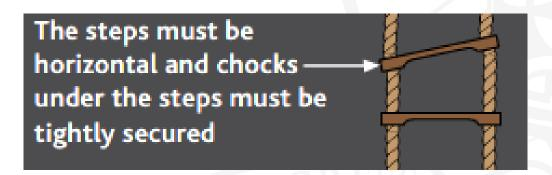
5.8. No pilot ladder should have more than two replacement steps and one replacement spreader.
