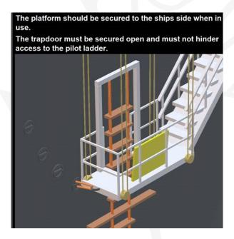
6.12. The pilot ladder should be secured to a strong point, independent of the pilot ladder winch reel by a rolling hitch:
