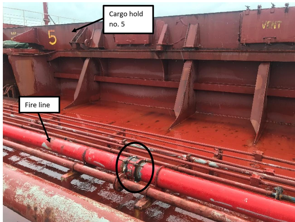
Figure 2: Location of the leaking flange on the fire line
