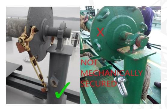
6.15. When a retrieval line is considered necessary to ensure the safe rigging of a pilot ladder, the line should be fastened at or above the last spreader step and should lead
