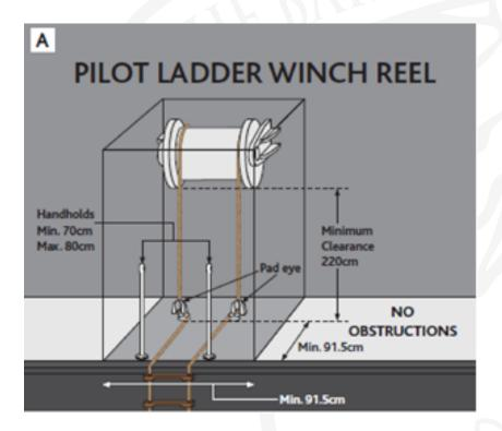
6.14. All pilot ladder winches should have means of preventing the reel from being accidentally operated as a result of mechanical failure or human error:
