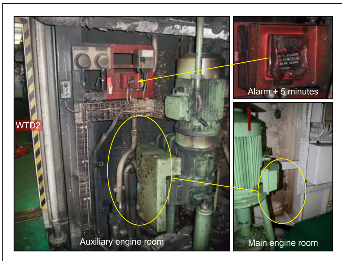
Damage caused by bilge fire
