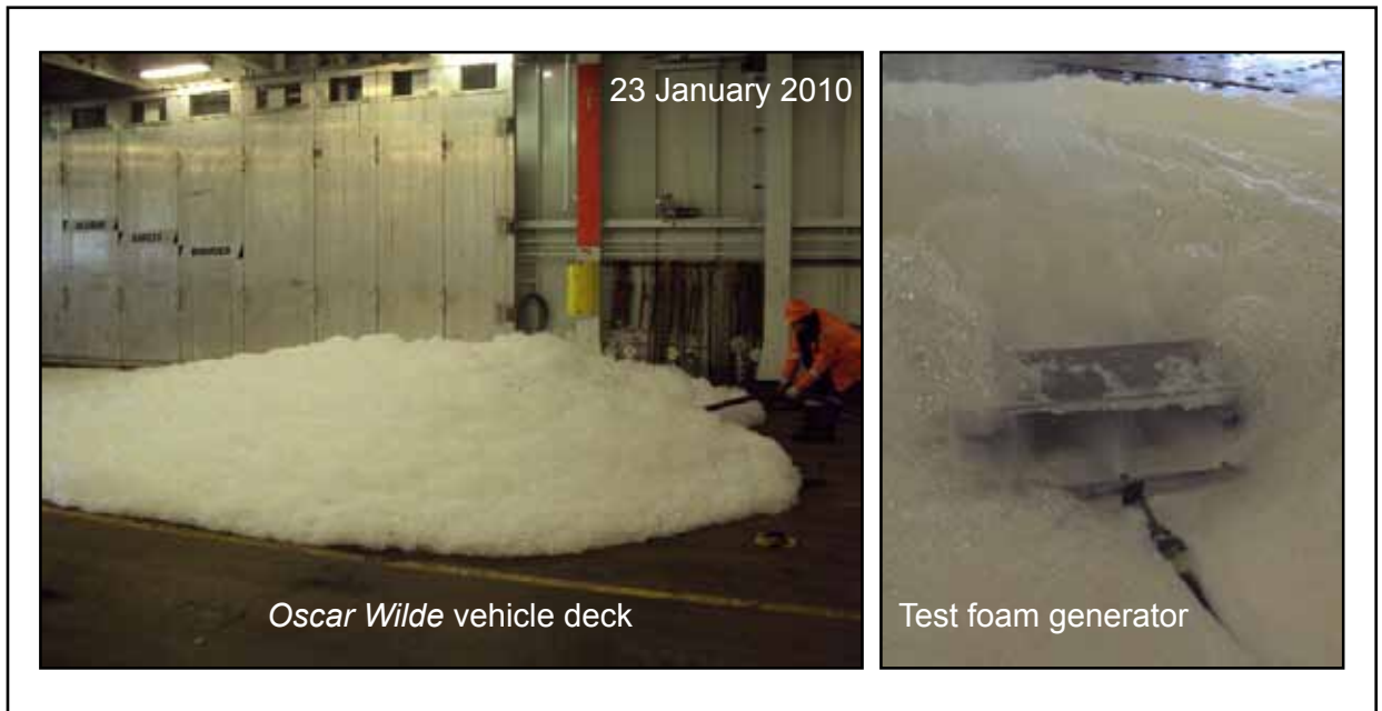
Hotfoam system discharge test
