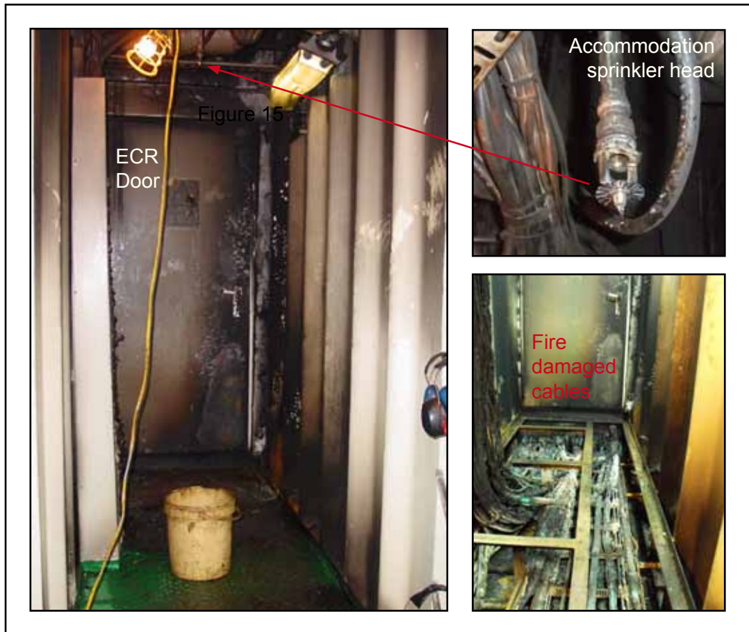
Fire damage on deck 2 outside the engine control room
