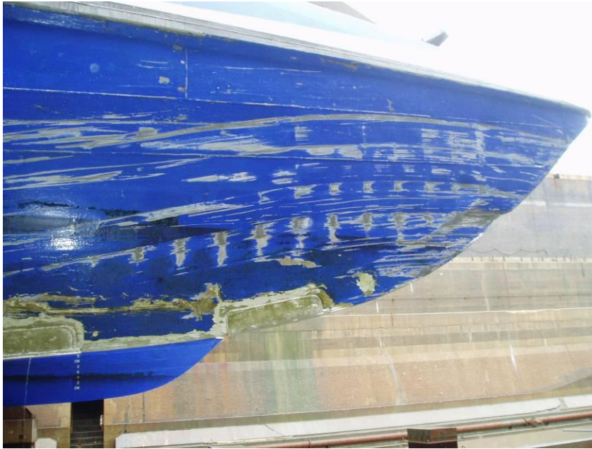
Figure 6: Damage to starboard bow of CONDOR VITESSE.
