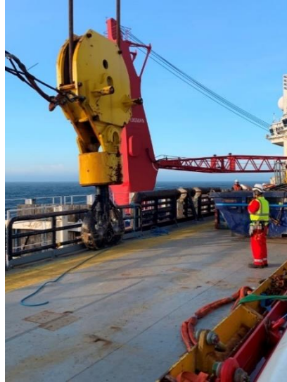
Figure 1: Location of the auxiliary block of the main crane secured to handrail
