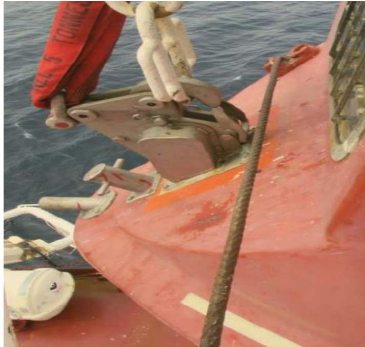
Figure 1: Aft gripe wire and hook mechanism
