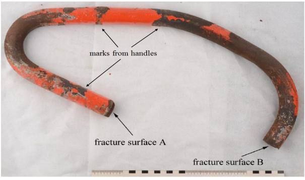
Figure 1: Fractured master link with handles removed
