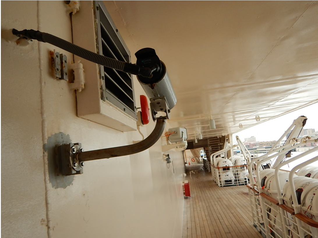
Figure 5: Camera view of stern blocked by floodlight (view looking aft on port side Deck 5)
