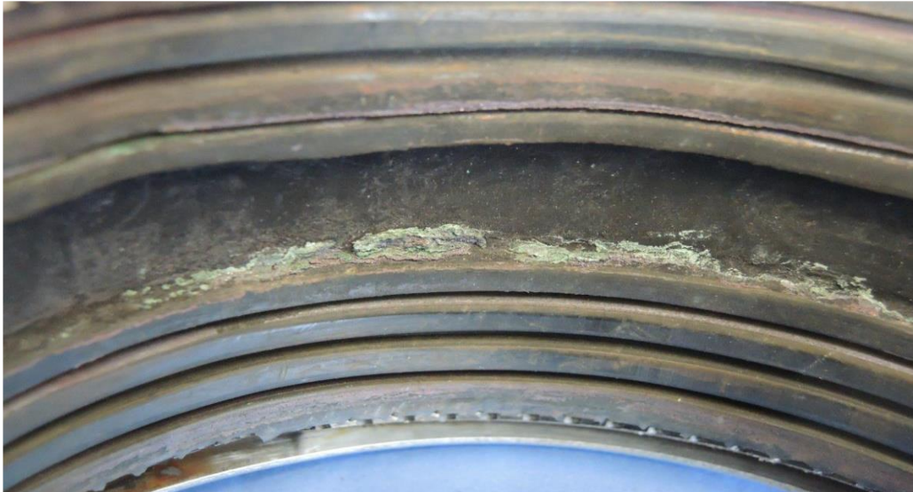
Figure 23: Greenish/turquoise deposit in the center of the gasket
