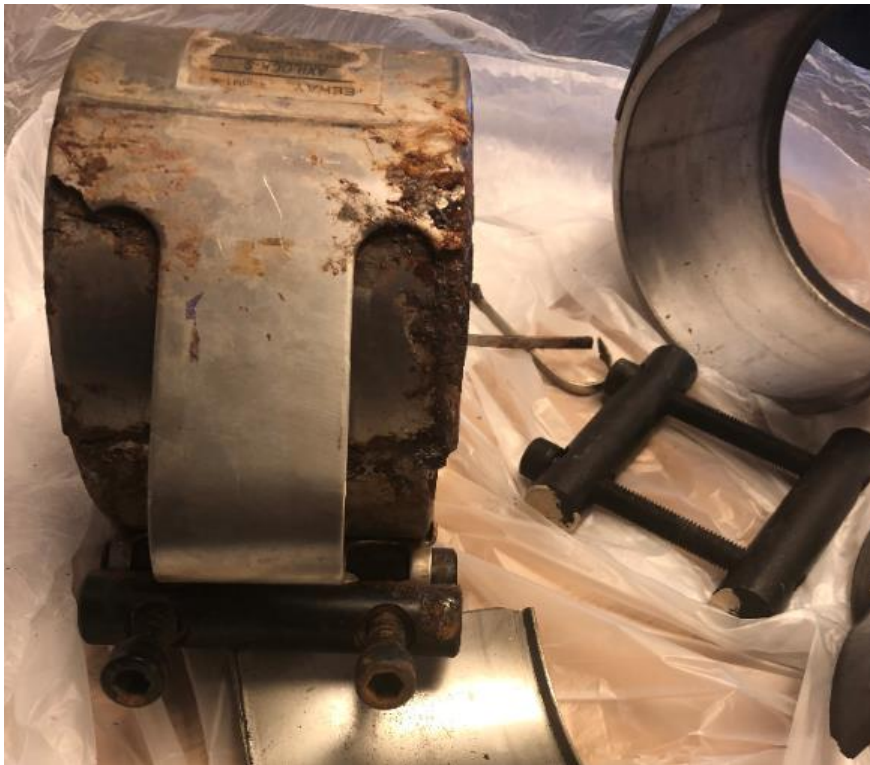
Figure 24: Failed coupling recovered after incident
