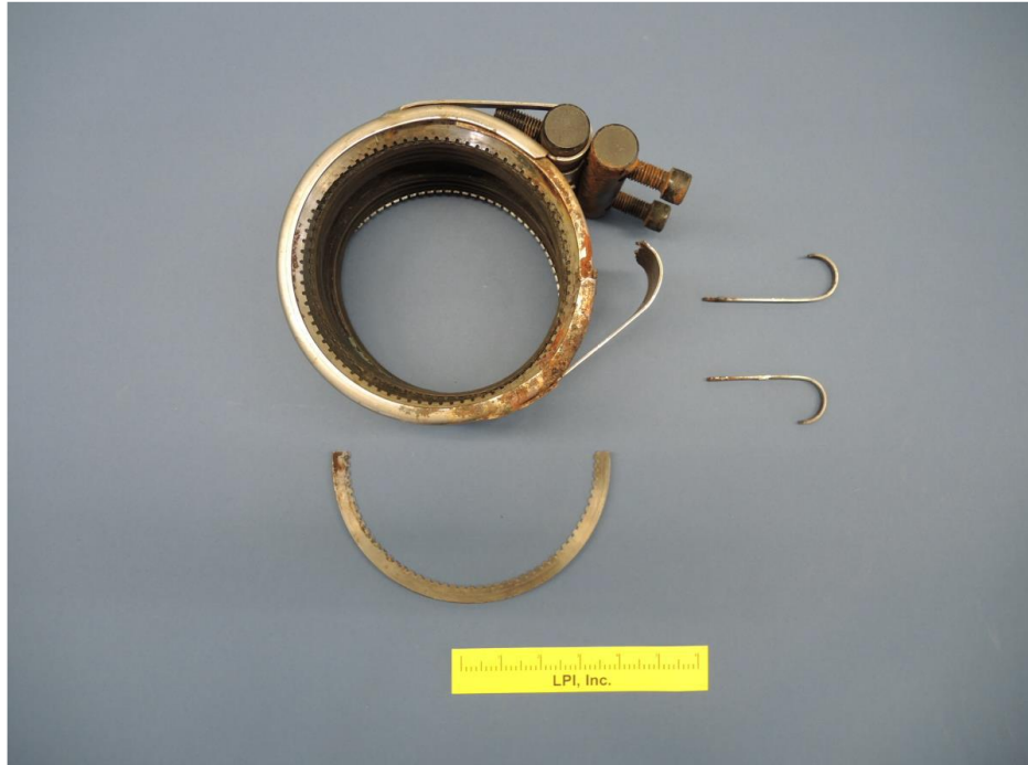
Figure 22: Failed coupling as received by LPI, Inc.
