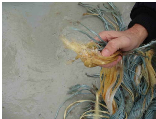
Figure 4.22: Above: Outer (blue) and inner (yellow and white) fibres have parted at the same position. Together with the fusing apparent on the inner fibres indications are that the parting of the rope depicted was very rapid.
