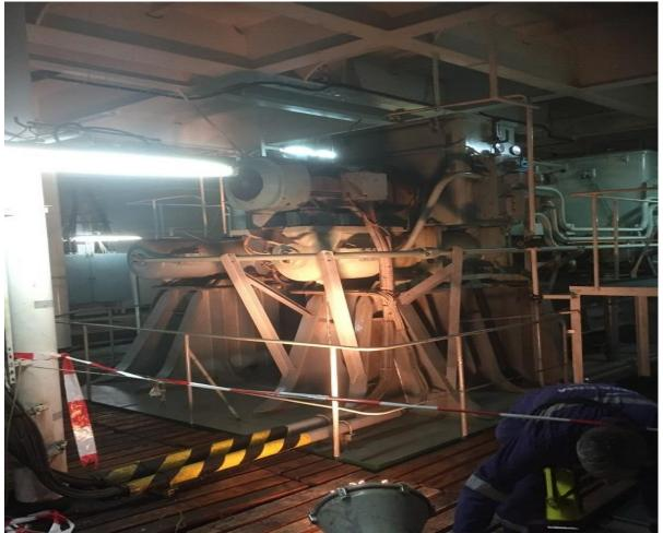
Figure 4: Foreman's view of stairwell access door obstructed by the steering gear
