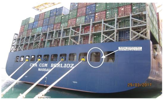
Figure 8: Vessel transom showing subject section of ship's side rails
