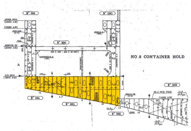
Figure 1: Structural cross section of vessel showing aft peak tank location highlighted in yellow
