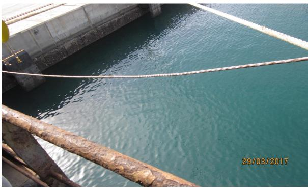
${\bf 2.}~{\bf Razor}$  wire rigging wire outboard of the aft rails
