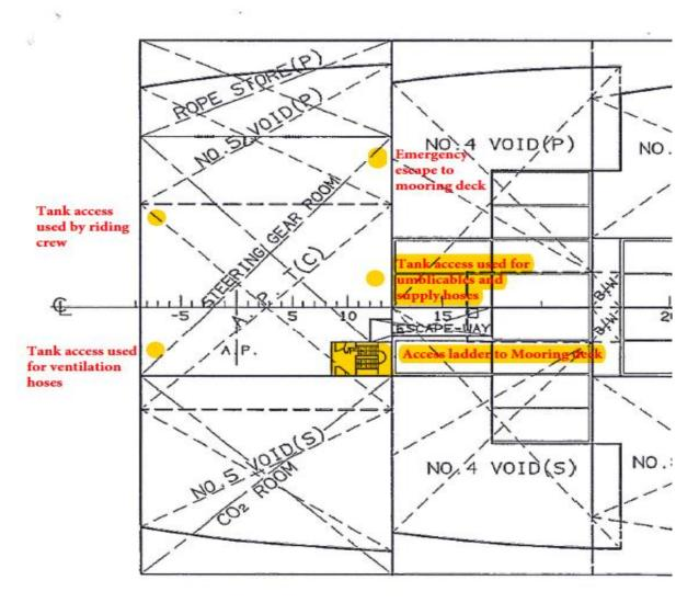
Figure 3: Plan view of steering gear room, aft peak tank, CO2 room and access points
