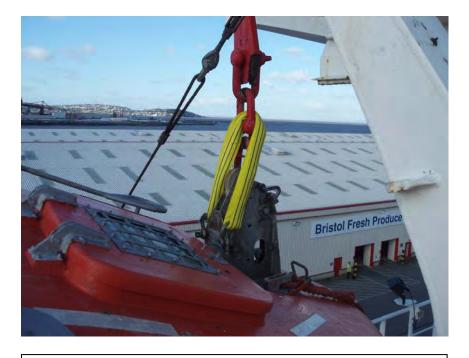
Continuous sling in place over-riding on-load release
