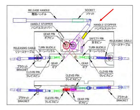
Figure 1: Release handle mechanism. Diagram from SHIGI Manual
