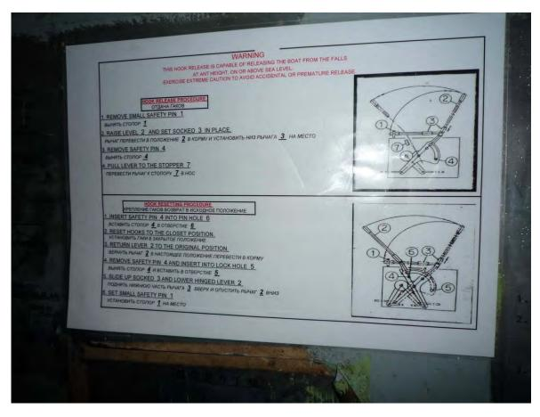
Photo 9: Instructions for Operation of the release mechanism and hook resetting procedure.
