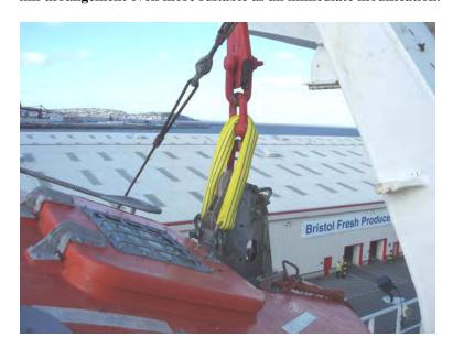
Note: Slings are more suitable as FPDs than are Strops as they do not have eye splices. This eliminates additional points of weakness. It also enables a shorter connection where this may be necessary.
