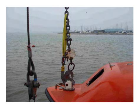
FPD taking load during exercise, simulating premature release of on-load hook. Note boat is not waterborne but suspended just above the water – a safety precaution for avoiding injury to personnel or damage to structures during the exercise. INTERNATIONAL MARITIME ORGANIZATION 4 ALBERT EMBANKMENT LONDON SE1 7SR
