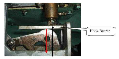
Photo 7: Under-deck Cam Plate in incorrectly re-set position.
