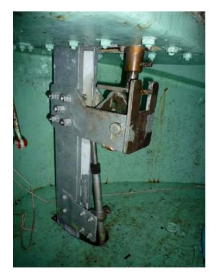
Photo 10: Underdeck Cam Plate visible for status check. Note this is incorrectly set.
