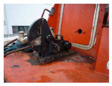
Photo 8: Hook as fitted. Note lug on side of side plate. There is another on the opposite side.
