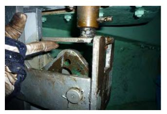
The under-deck Cam Plate indicating a position in which the release of the hook was possible (not necessarily the position in which the failure occurred but held in this position for clarity of subject area )
