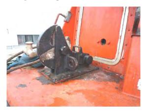
Above and Right: After hook arrangement on the SHIGI boat showing side lugs that are suitable points of attachment for FPD Slings.as in the arrangement below.
