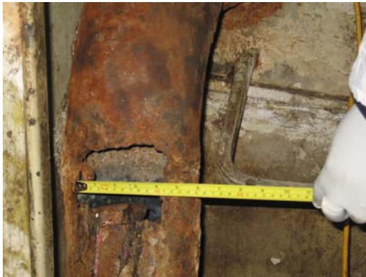
Hole in overboard pulper pipe. Width approximately 4 1/2 inches.
