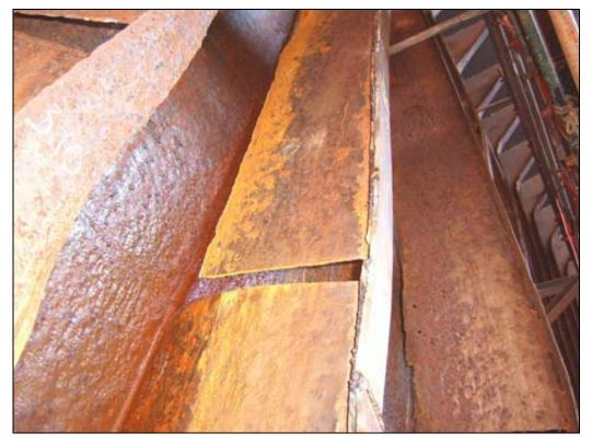
Cargo hold No.1 – Port side frames 310 and 311, corroded, tripped and detached.
