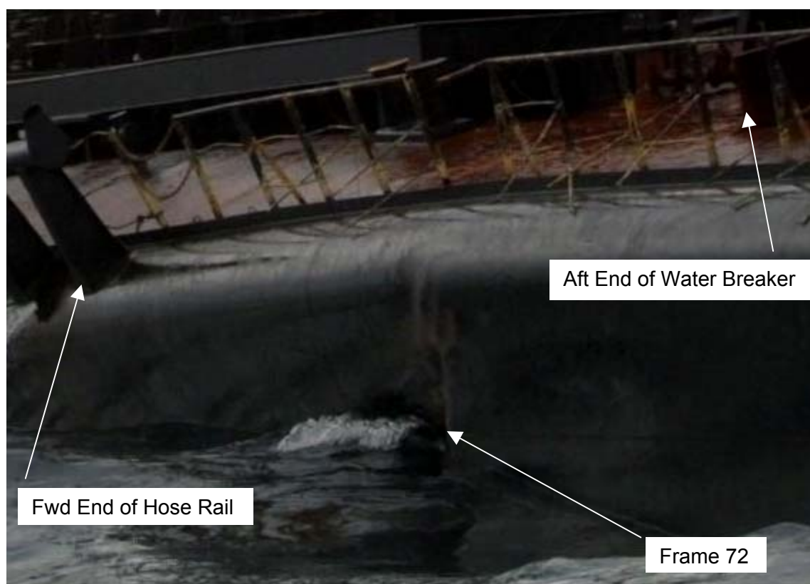
Forward most deformation of main deck edge and side in way of 3 Starboard Ballast Tank and 2 Starboard after wing tank
