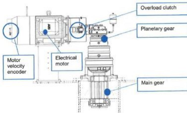
Figure 4: Steering motor unit parts (source: AN Propulsion Study report by ABB, DNV-GL, Elomatic, MeyerWerft, RCCL, VTT)
