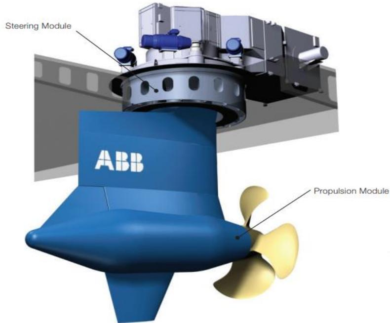
**Figure 2: Basic arrangement of the Azipod (Source: ABB website)**
