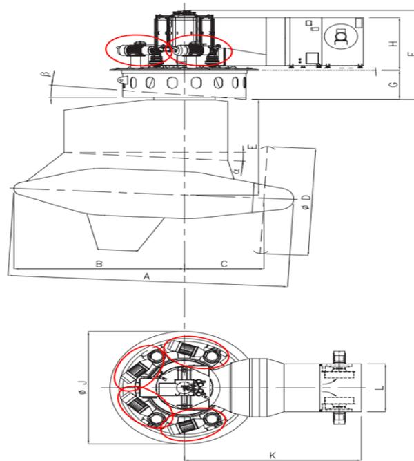
Figure 3: Motors arrangement on Azipod highlighted in red circles
