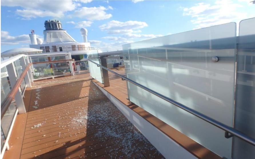
**Figure 10: Broken glass on deck**
