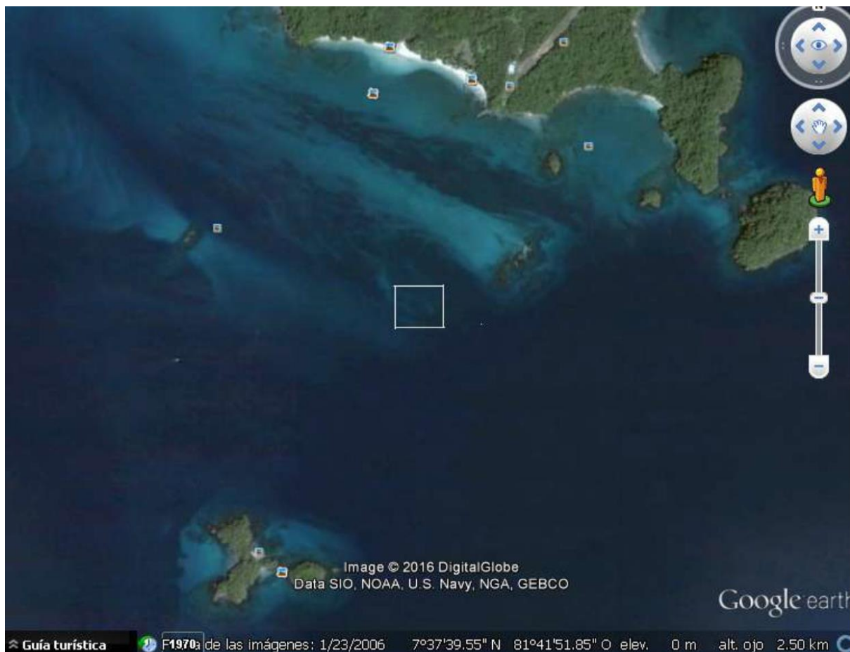
Figure 21: Google Earth image with a white box around lighter blue water at the grounding location, indicating visually an area of shallow water
