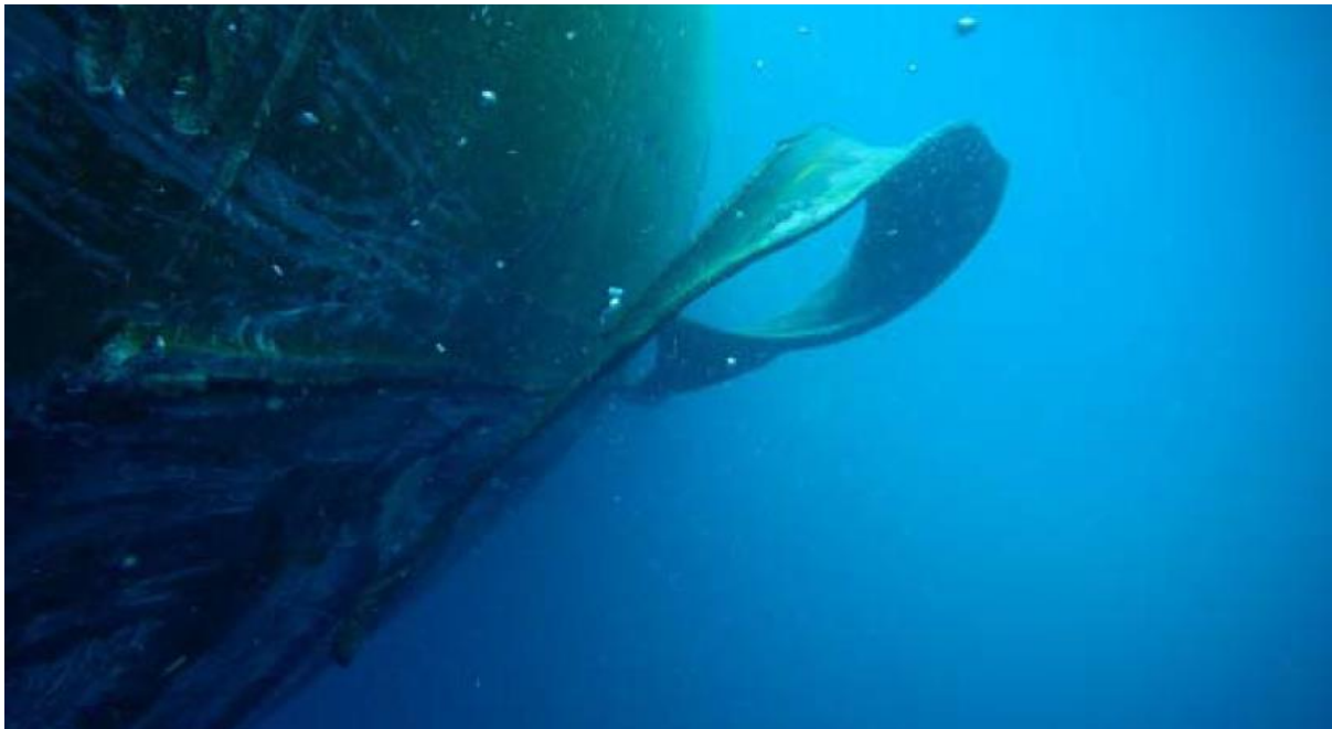
Figure 17: Bilge keel port side partially detached from vessel
