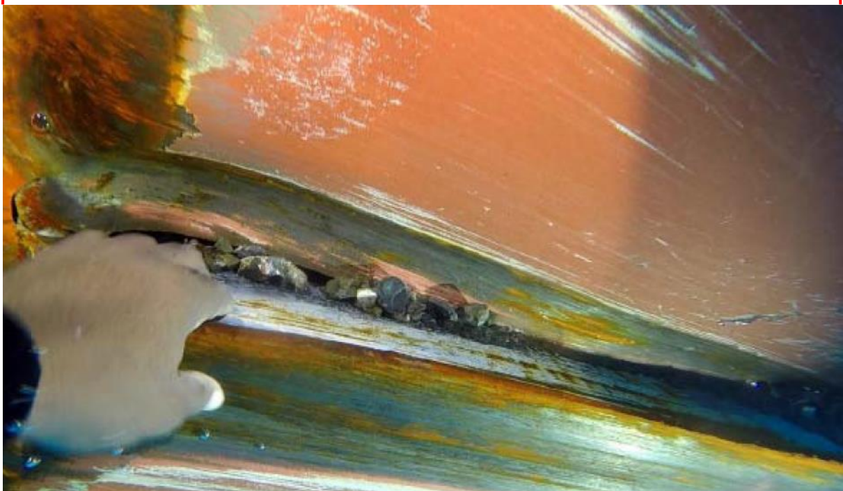
Figure 12: Frame 92 – 95 port centre, longitudinal crack 1800mm x 80-120mm in way of #3 port grey water tank
