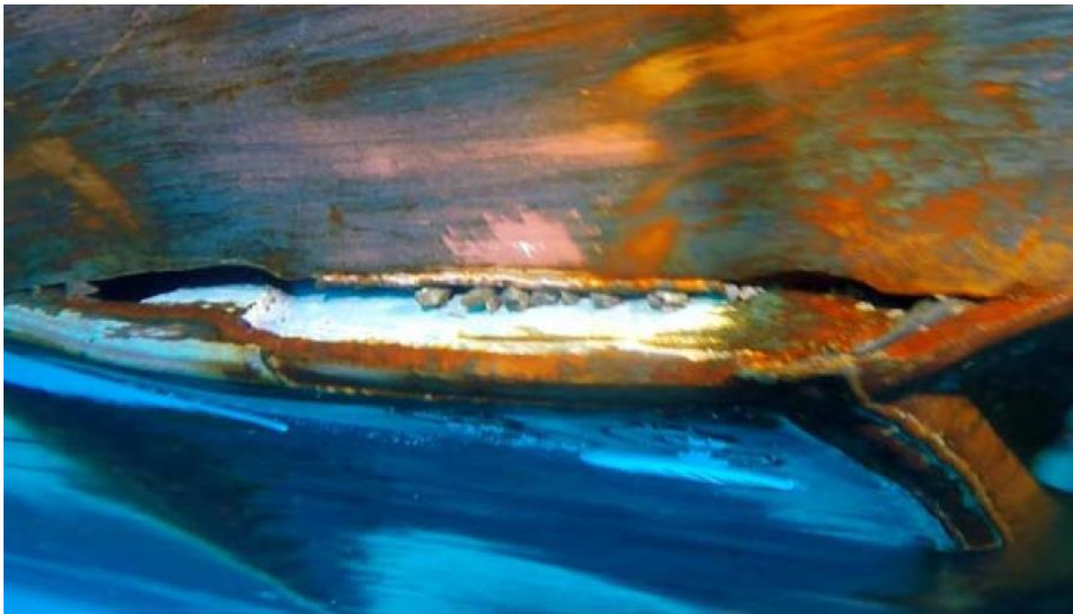
Figure 13: Frame 82 – 86 starboard side, longitudinal crack 400 x 60-80mm in way of #3 starboard grey water tank and #5 centre MGO tank, 2 nd crack 105mm x 30-40mm in way of #3 starboard grey water tank and #5 centre fuel oil tank
