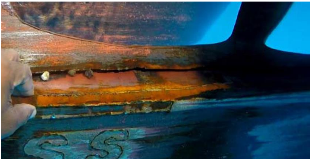
Figure 15: Frame 63-66 starboard, 100-150mm indentations below starboard stabilizer. Crack 1500mm x 60-80mm into #6 HFO tank. Crack 100mm x 10mm into #15 starboard FO overflow tank.
