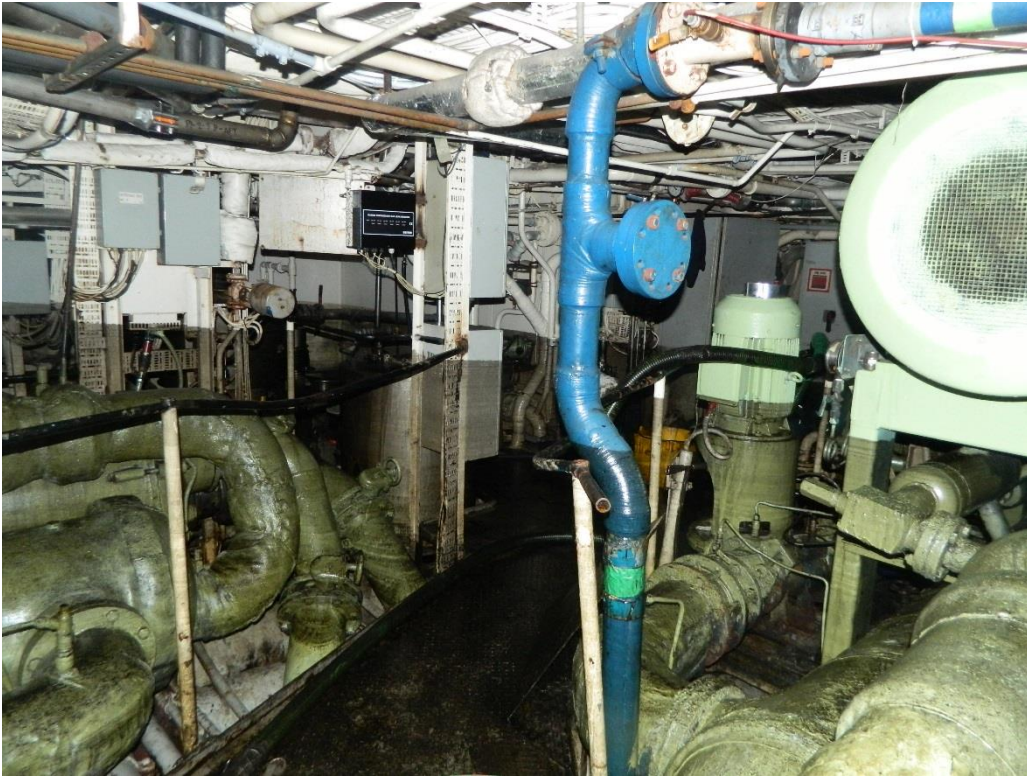
Picture 5: The forward engine space at Balboa anchorage after tow (the dark stain indicates the maximum depth of flooding)
