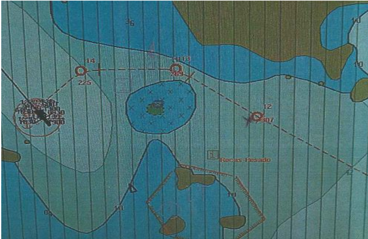
Figure 19: Reproduced ECDIS screenshot with 'x' marking the position of the unknown source of the bumping experienced on the 16 th December
