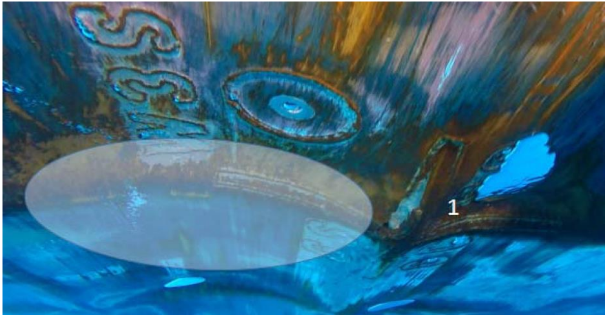
Figure 14: Frame 75 port side, 50-100mm plate indentation/deflection under tank 6 port and 7 port HFO/sludge storage tanks. No cracks. Frame 84 (image not shown) minor indents.
