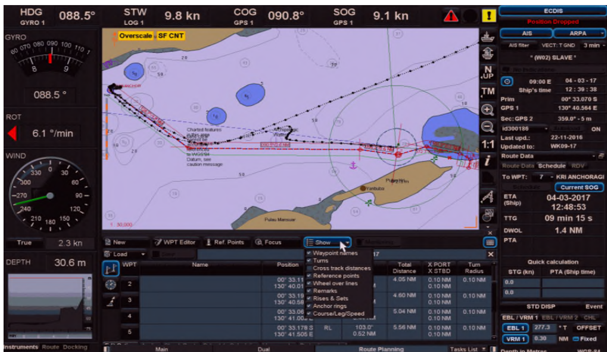
Figure 4: ECDIS screenshot taken moments prior to the grounding at 1239
