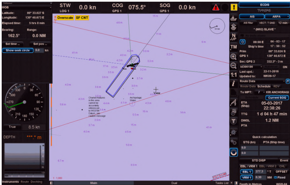
Figure 7: ECDIS screenshot displaying results of soundings taken in proximity to the vessel
