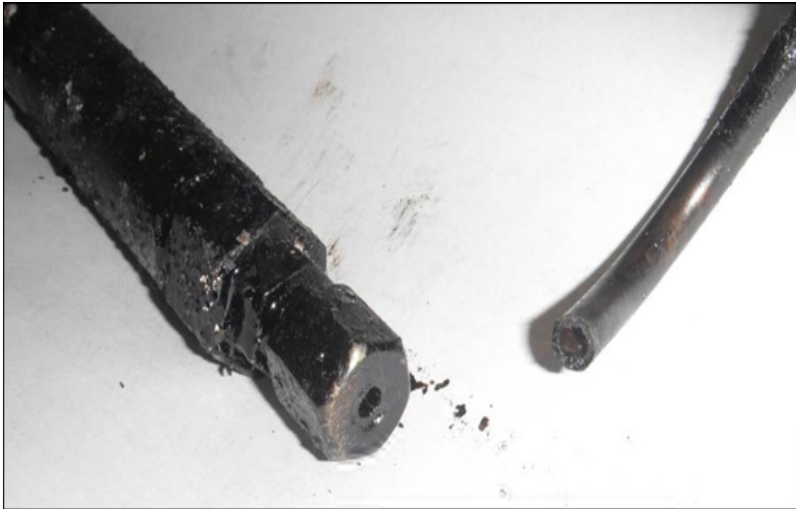
Figure 11: Point of fracture in the fuel oil pressure gauge supply line
