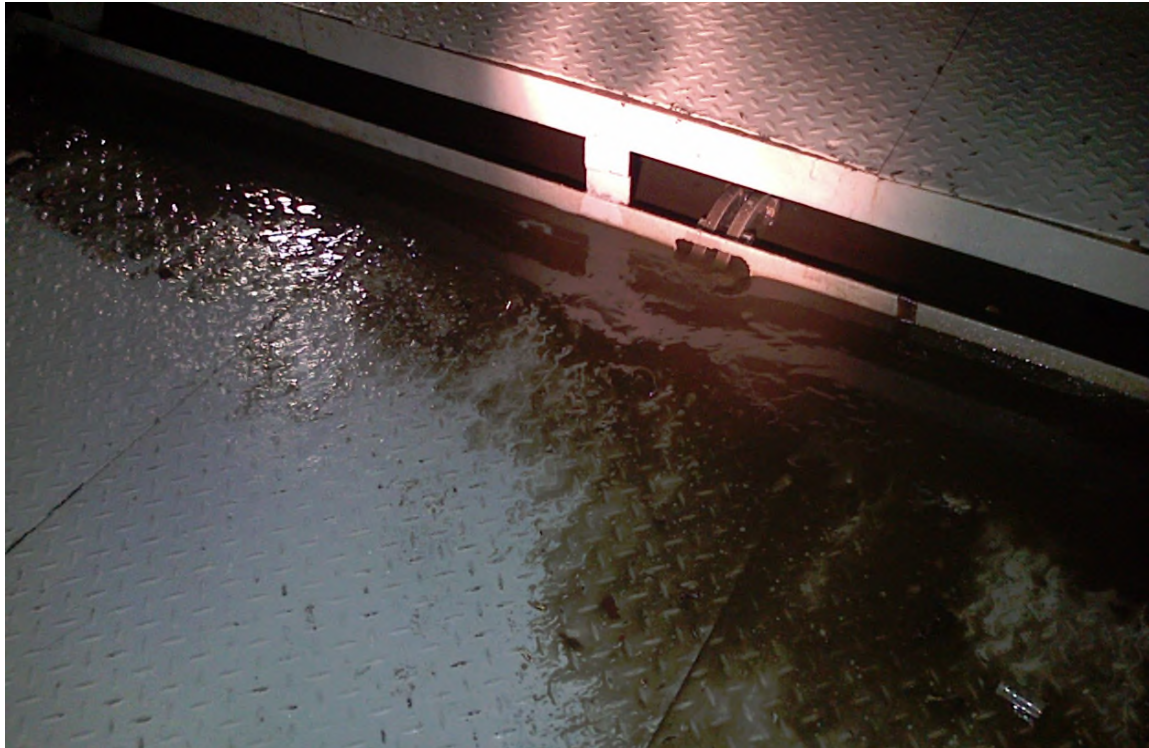
Figure 25: Mid tunnel tank top flooding (Frame 40-60)
