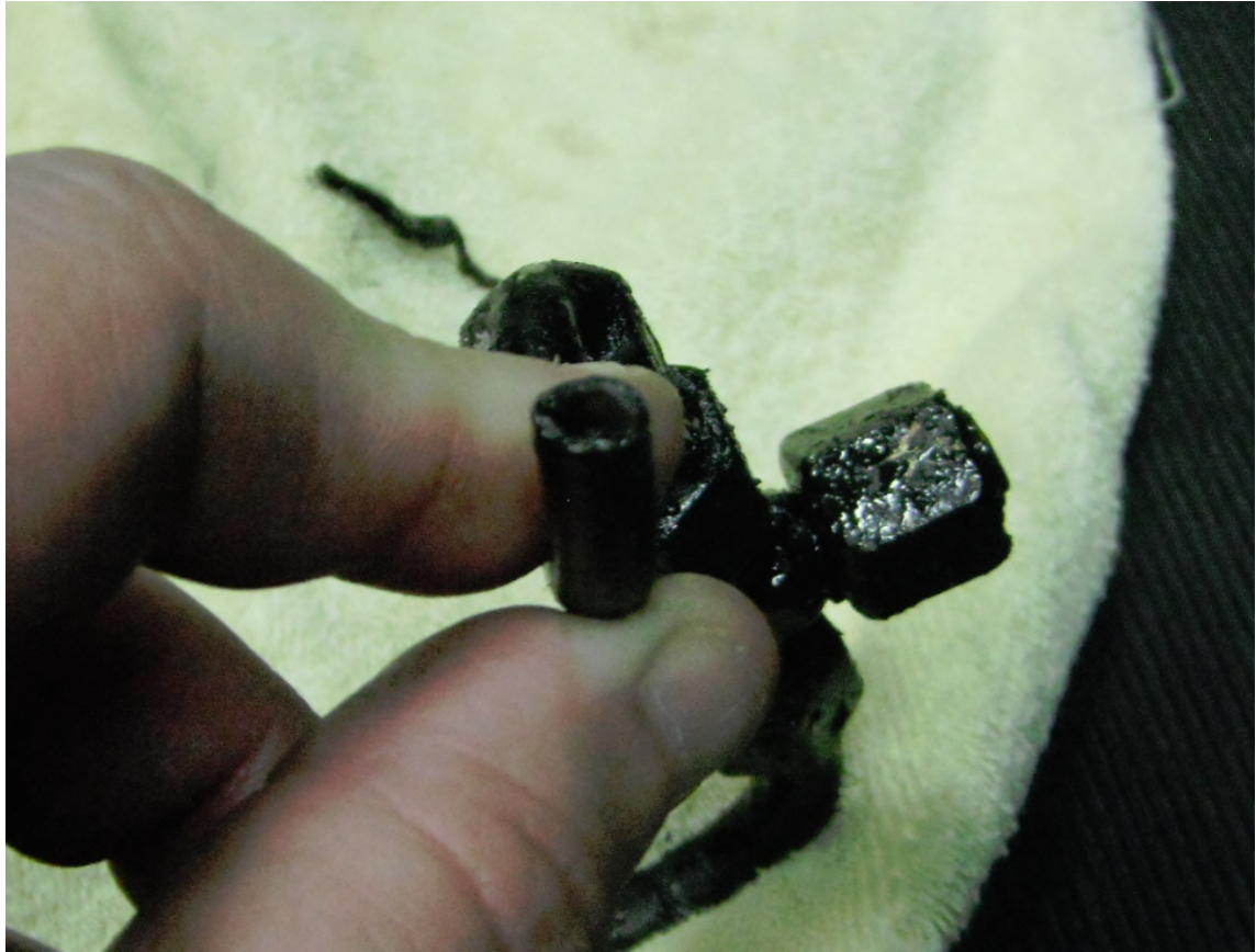
Figure 27: Fractured fuel oil pressure gauge supply line
