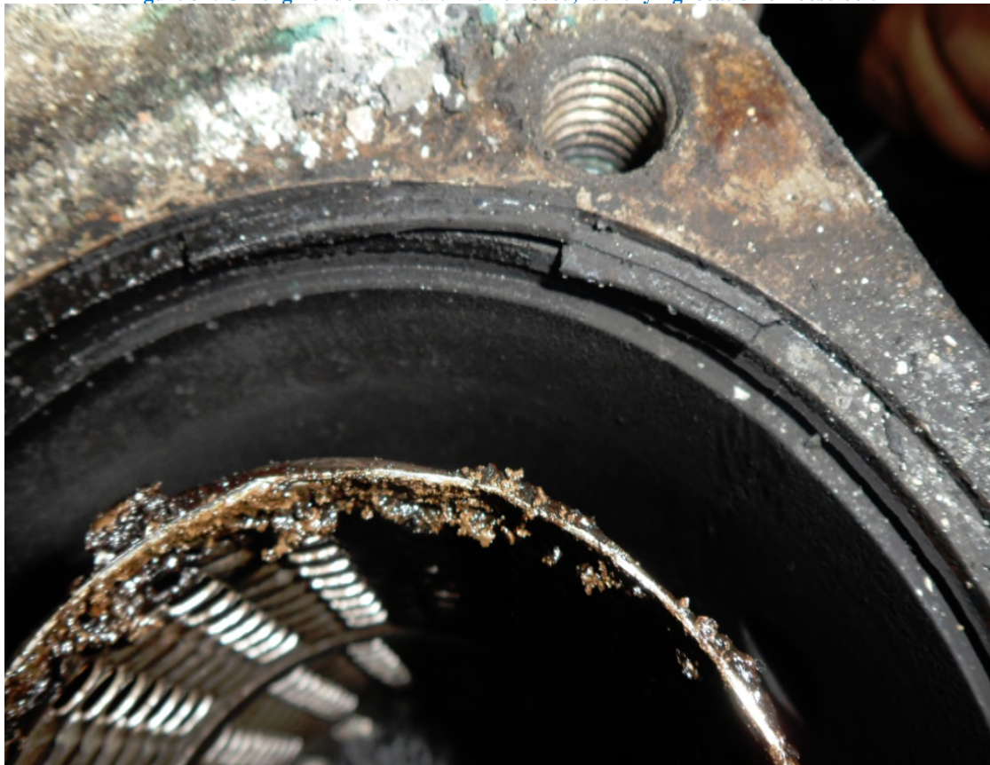
Figure 35: On-engine fuel filter damaged seal with lid removed
