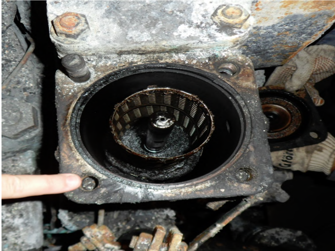
Figure 34: On-engine fuel filter with lid removed, identifying location of loose bolt
