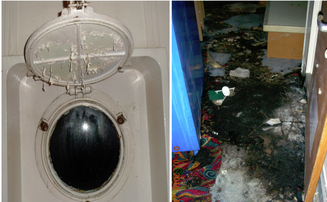
Figure 27: Heat damage sustained in cabin 311 above the seat of the fire
