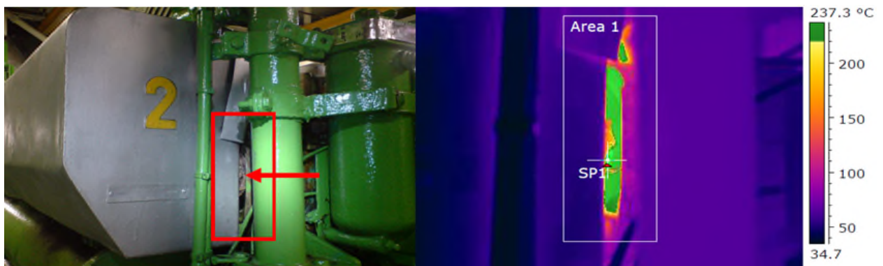
Figure 16: Temperature of 355.3°C in vicinity of exhaust manifold (highlighted left) and SP 1 (right)
