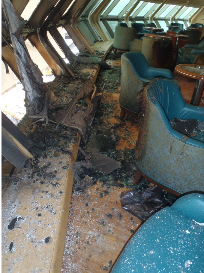
15 Fire Damage in the Deck No. 6 Aft Lounge
