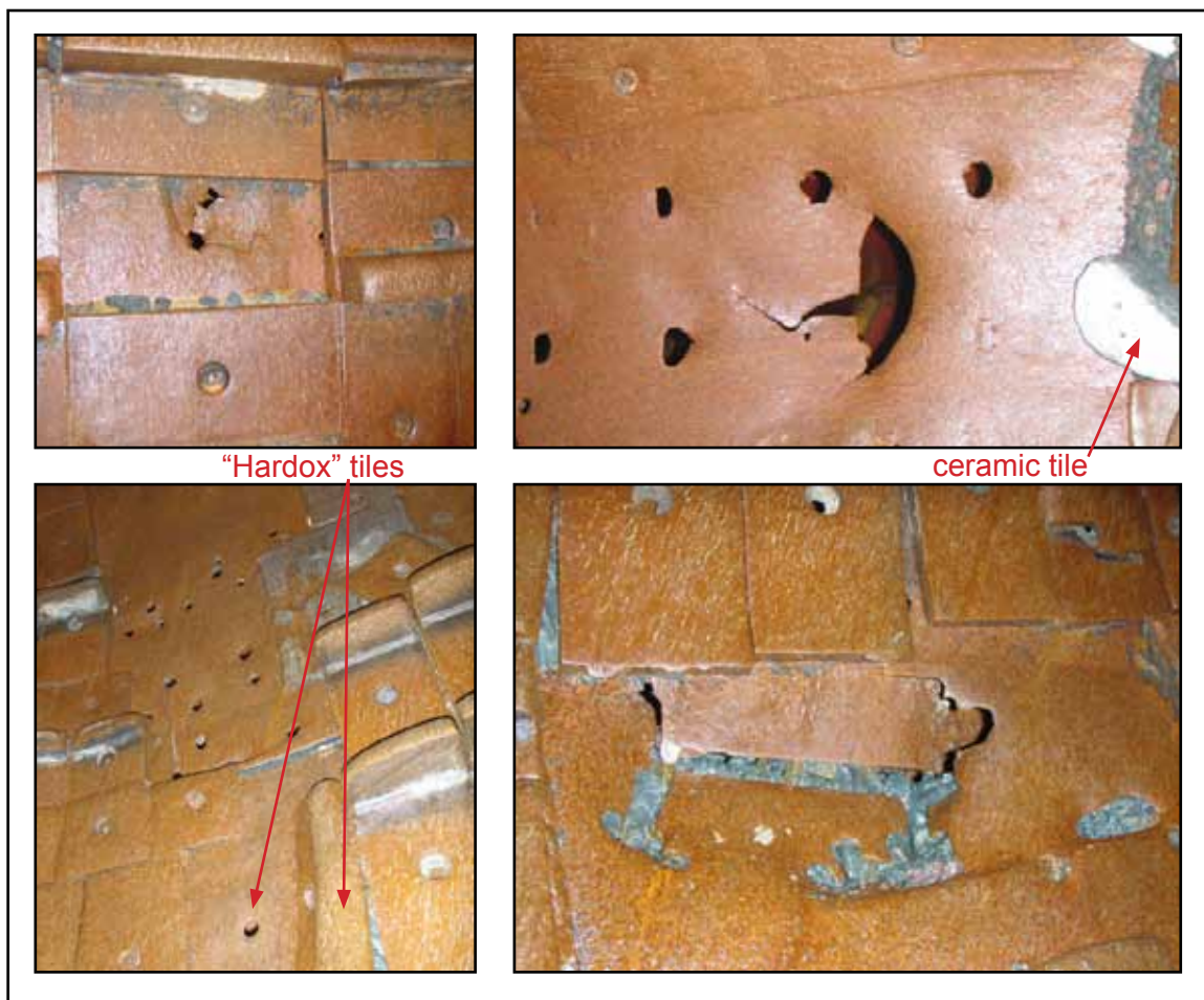
Composite of photographs showing discharge hopper damage and wear to the "Hardox" and ceramic sacrificial protection tiles
