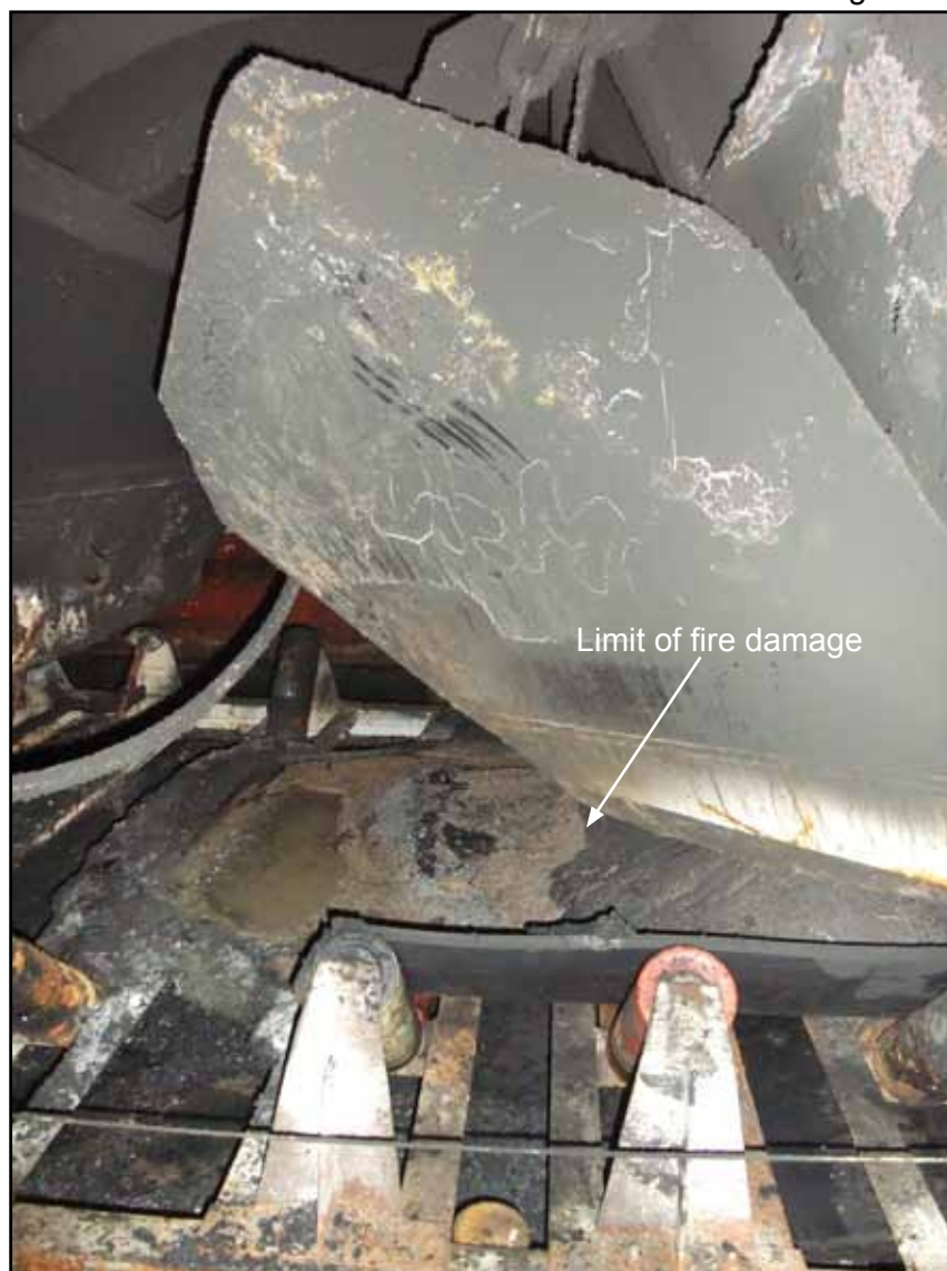
Extent of damage to tunnel conveyor belts
