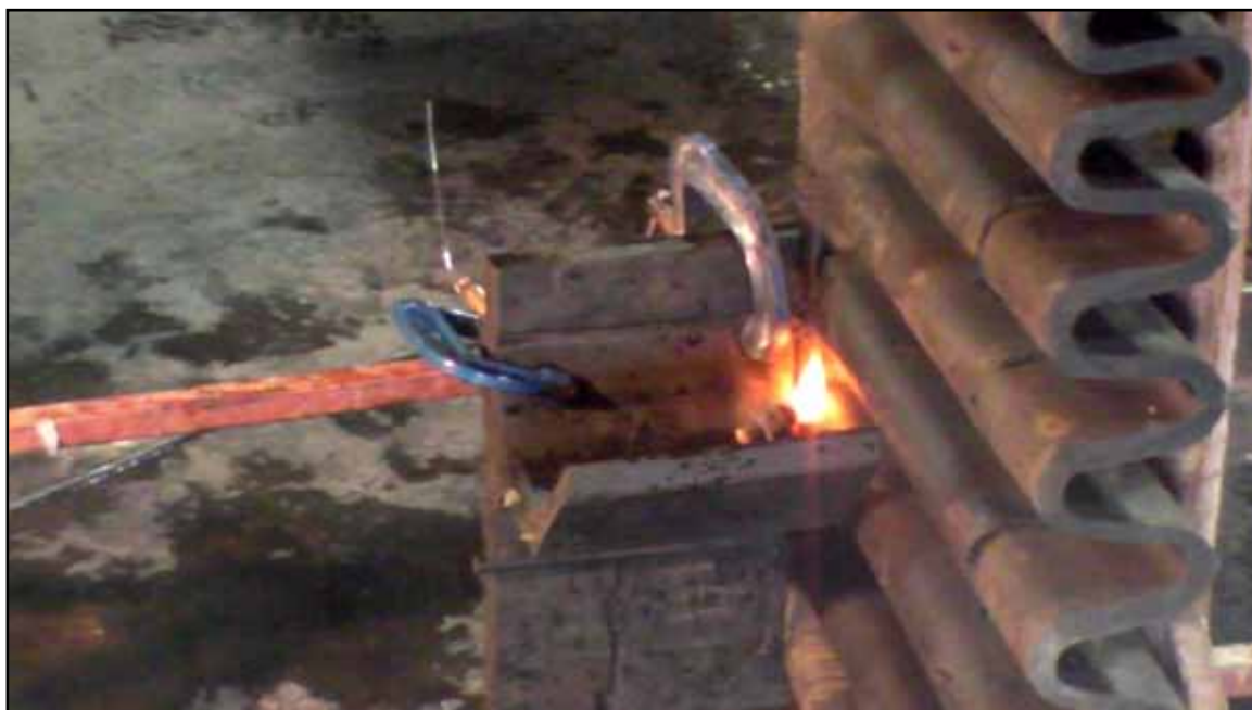
Fire Tests - stud and nut placed in cleat adjacent to the side curtain
