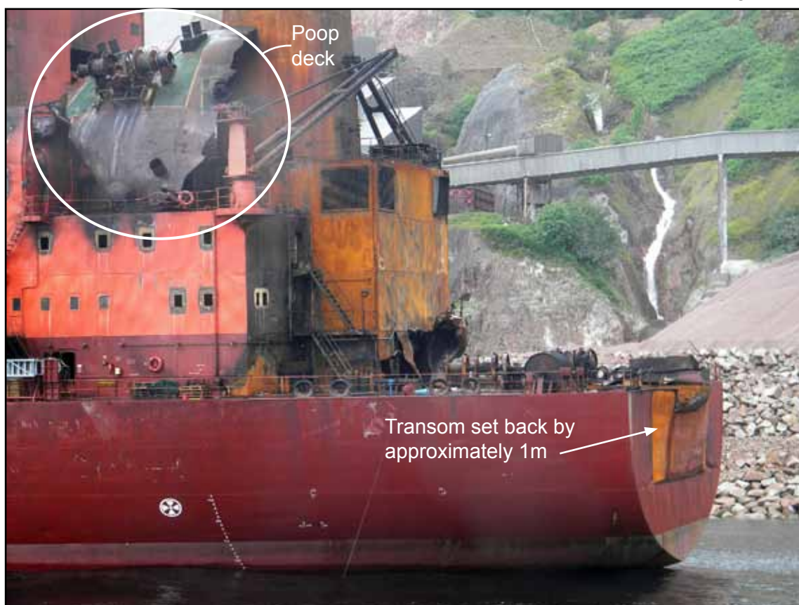
View of poop deck relocated to the funnel deck
