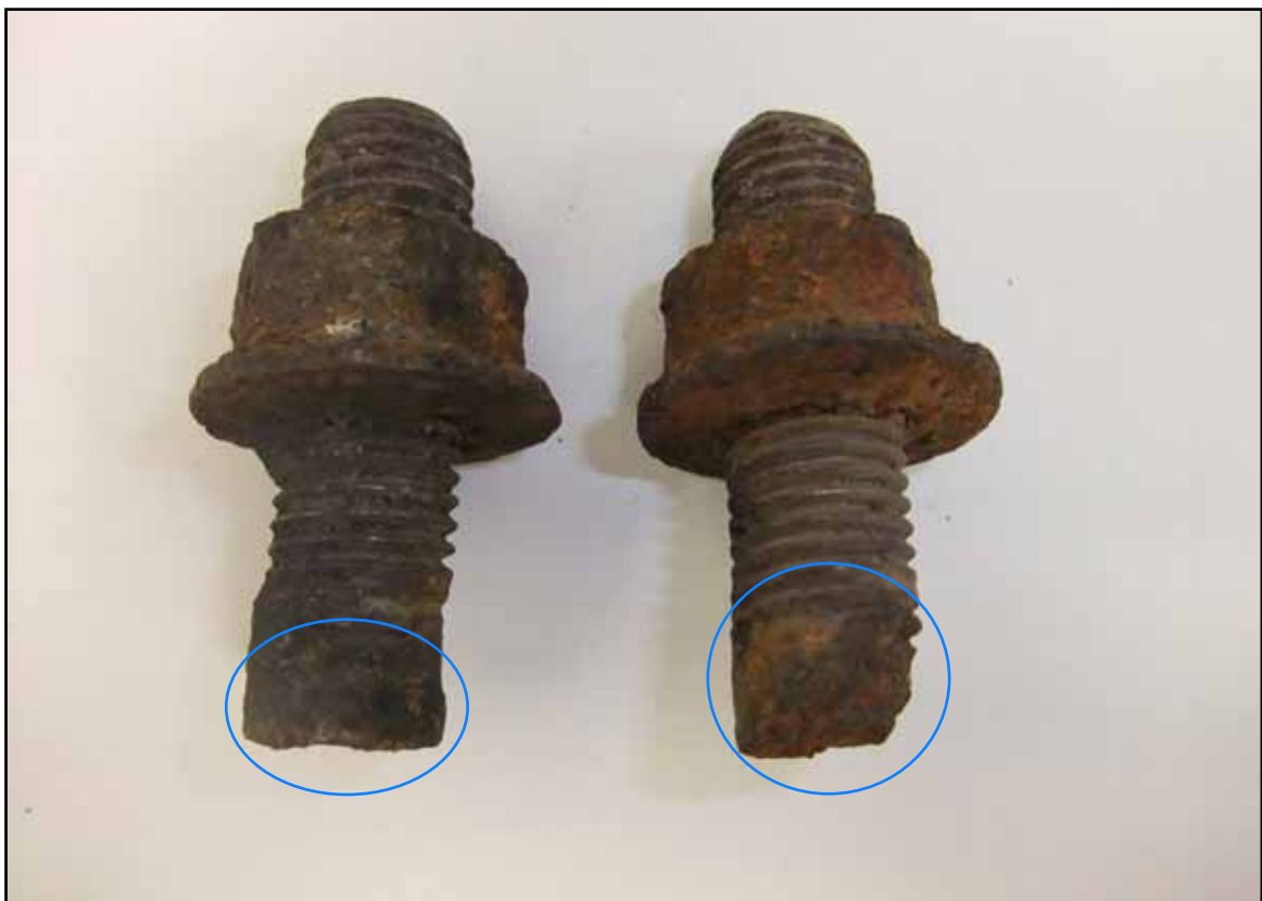
Flame cut bolts similar to those used to secure the "Hardox" tiles
