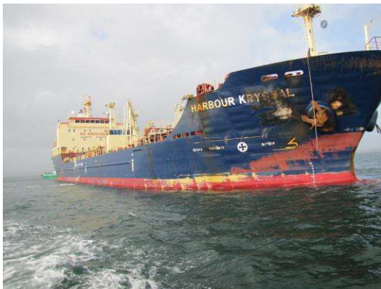
Hull damaged with burning marks
