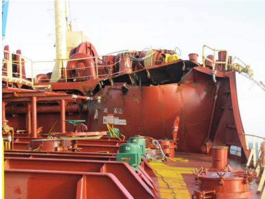
Bulkheads pushed outwards due to explosion pressure
