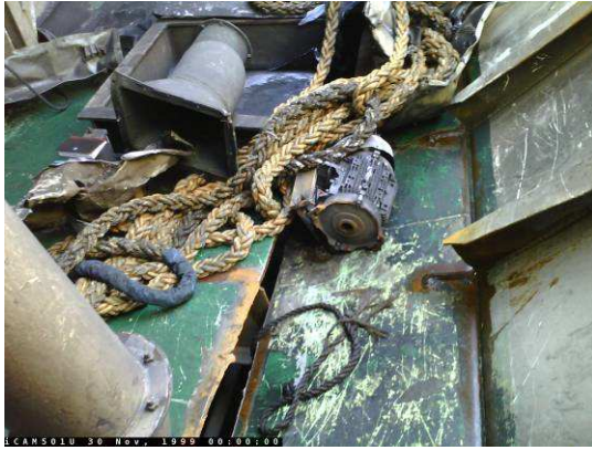
Deck pushed and broken. Motor from de-humidifier
