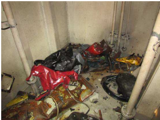
Aft bulkhead buckled towards the aft. Plastic affected by heat
