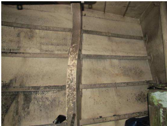
Distorted Hull frame
