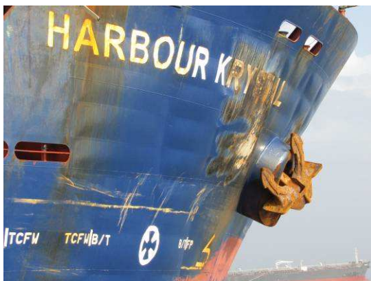
Hull buckled between frames and reinforcements
