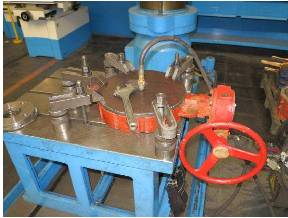
Isolating valve under testing
