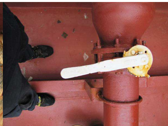
Isolating valve in closed position but in line with colours Tank valve in closed position not at right angle to line
