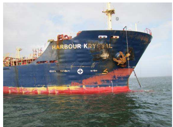
Hull damaged with burning marks
