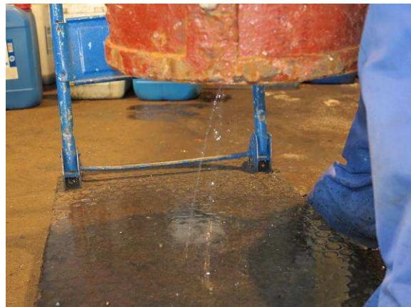
Non-return valve heavily leaking without pressure
