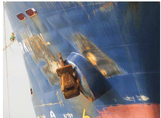
Hull buckled between frames and reinforcements
