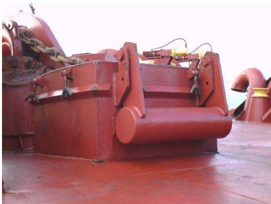
Forward port square hatch missing. Ripped out from counter weight
