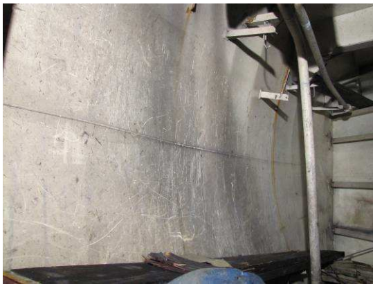
Aft bulkhead buckled towards the aft
