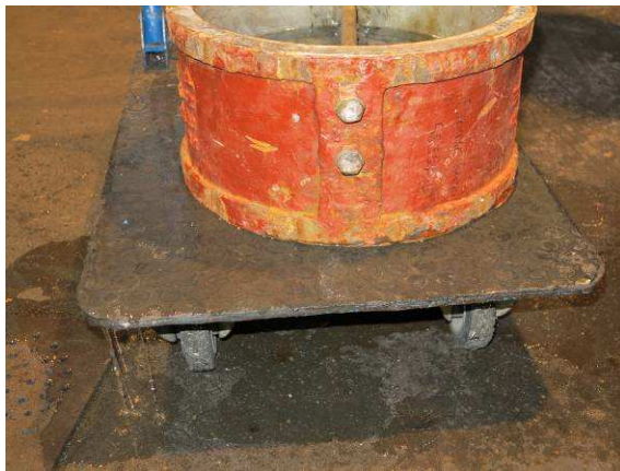
Non-return valve heavily leaking without pressure
