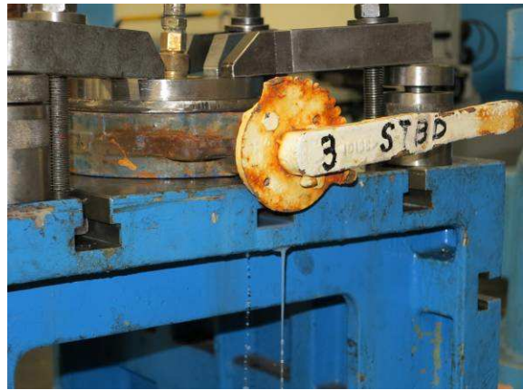
Tank valve leaking during test
