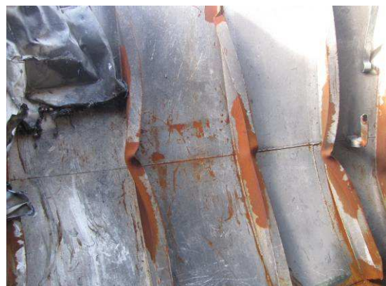
Aft bulkhead pushed outwards
