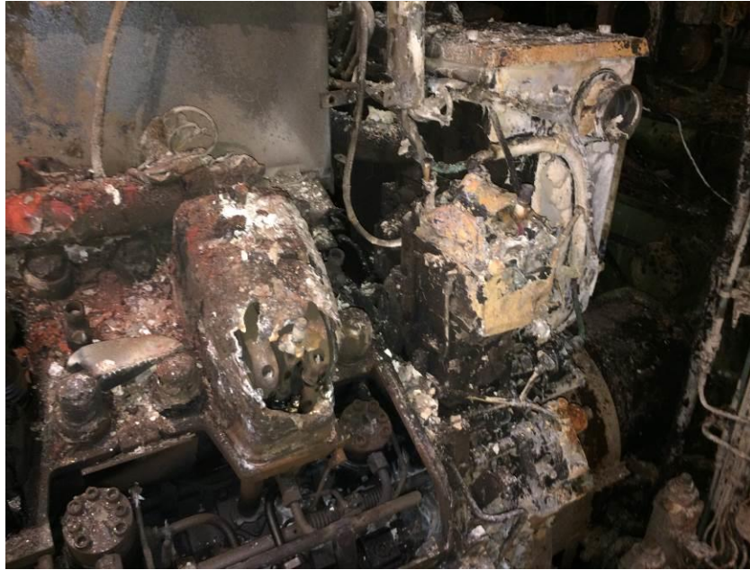
Figure 31: Fire damage to the aft section of starboard main engine
