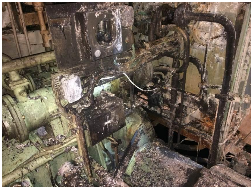
Figure 32: Damage to the area in way of starboard gearbox and oil cooler
