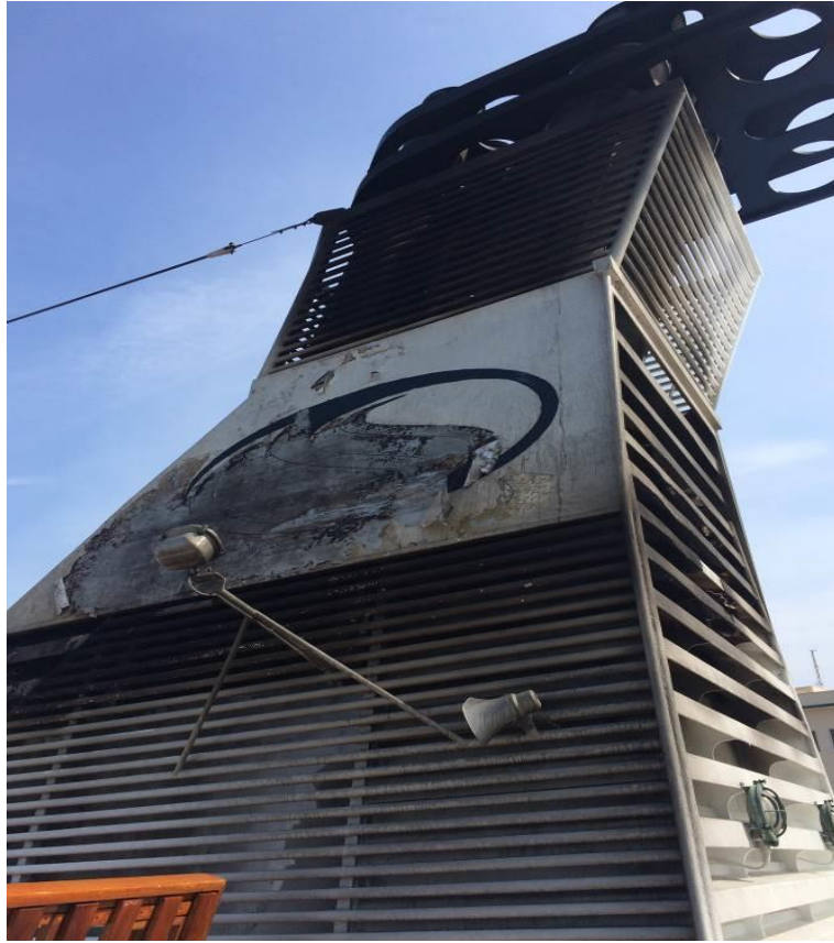
Figure 29: Heat and smoke damage to Portside funnel
