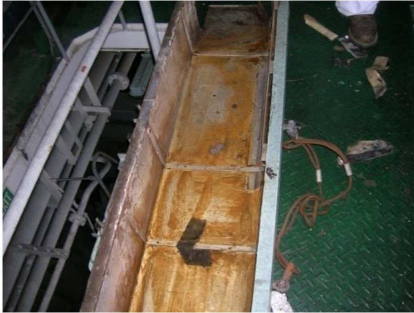
Figure 14: The No. 3 generator exhaust manifold cover not in Position
