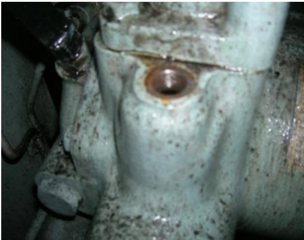
Figure 10: Location of probe on lube oil system
