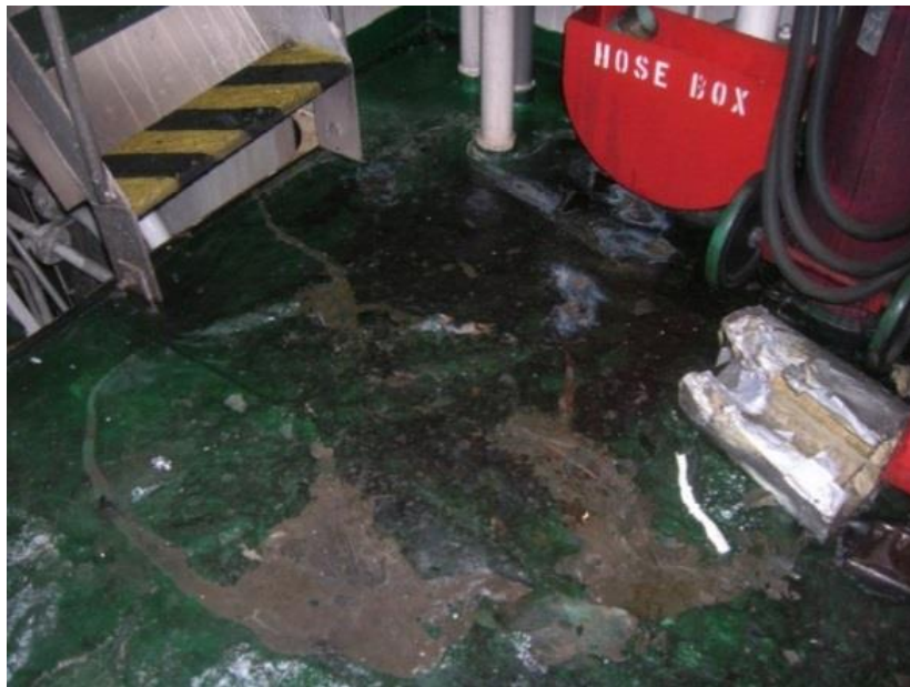
Figure 21: Deck above workshop buckled due to heat
