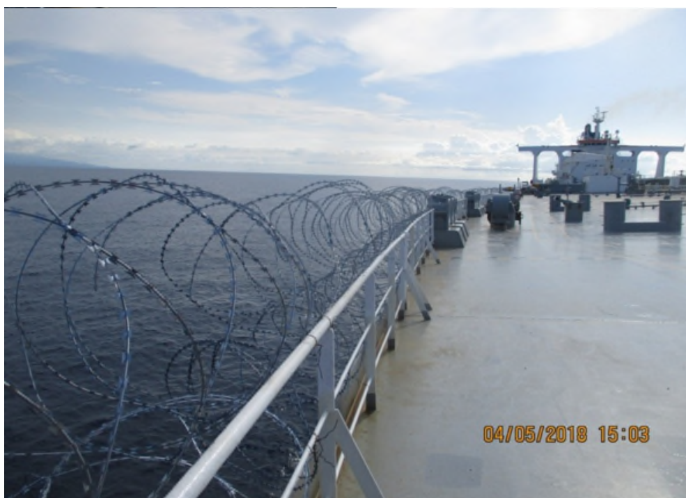
Figure 3: Starboard side razor wire in place as a self-protective measure against threat of unauthorised boarding
