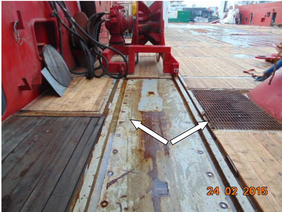
Figure 5: Chain hauler guide rails
