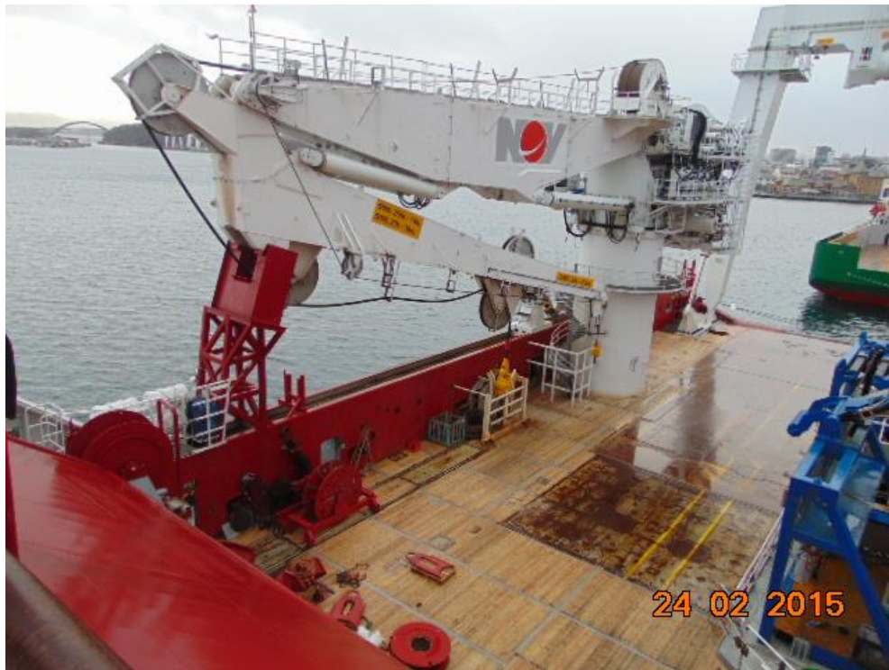
Figure 4: Crane (20-tonne) for lifting Gypsy
