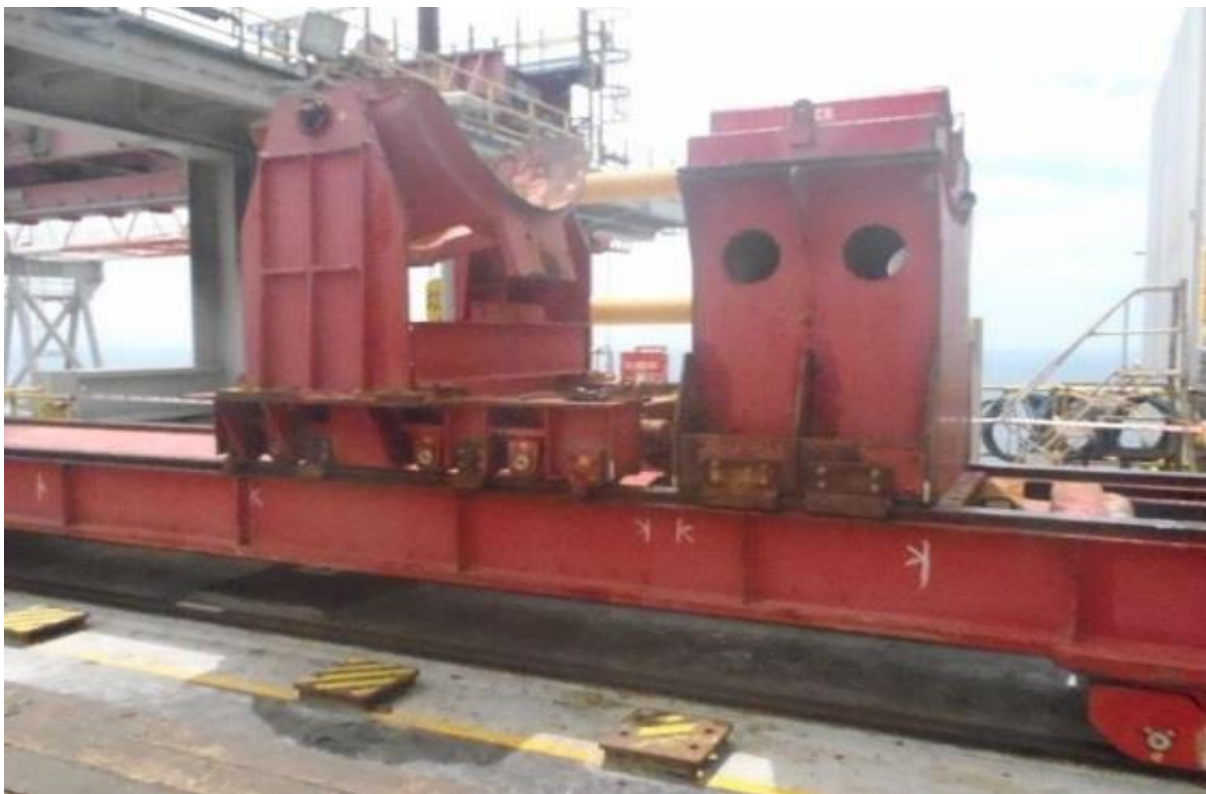
Figure 5: Starboard side view of support trolley (left) next to riser support lower cradle (Right)
