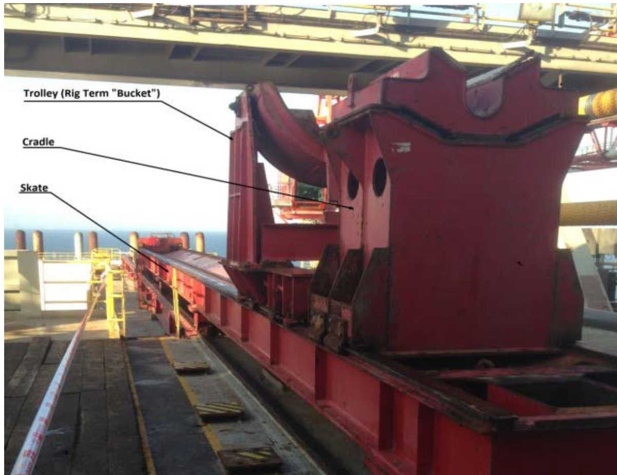
Figure 3: Starboard side view of Riser Feeding Machine looking aft
