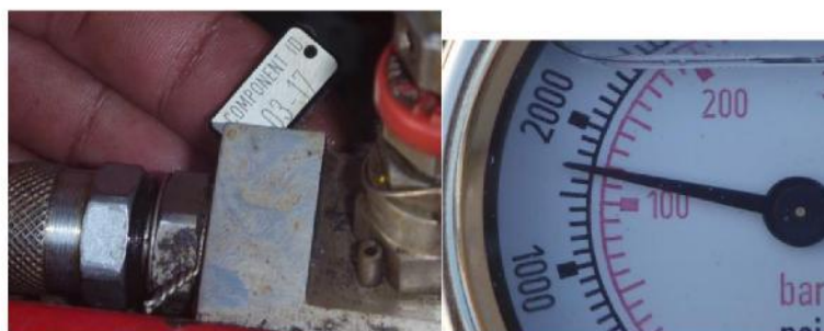
Pressure reading 125 bar, from port ID 03-17. Refer to drawing 3285263.
