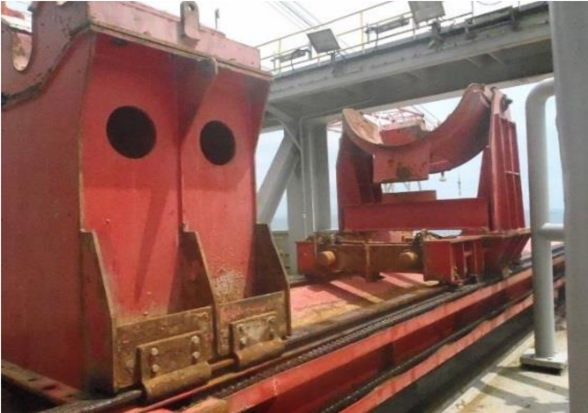
Figure 4: Port side view of Riser Feeding Machine with support trolley (bucket) aft with riser support lower cradle in foreground
