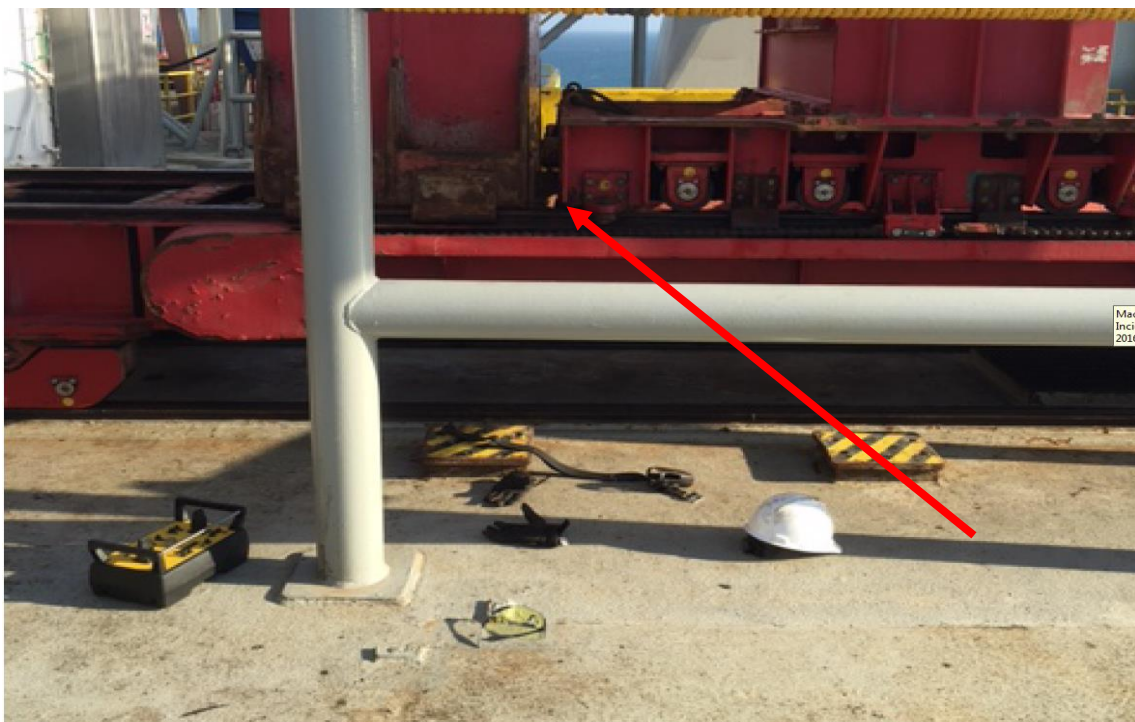
Figure 24: Location of PPE, RCP and stopped position of the riser support and trolley, gap indicated by arrow
