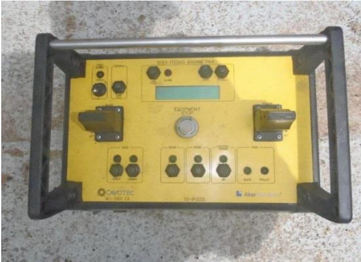
Figure 8: Remote Control Panel (RCP) for operating the RFM
