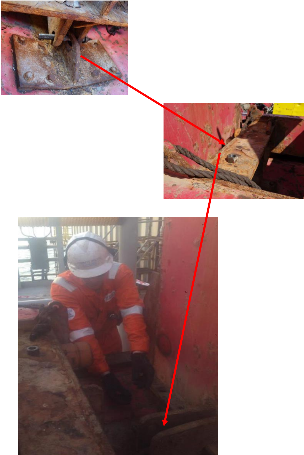
Figure 29: Images depict the process considered to possibly undertaken by the Trainee Driller at the point of impact between the riser support and trolley
