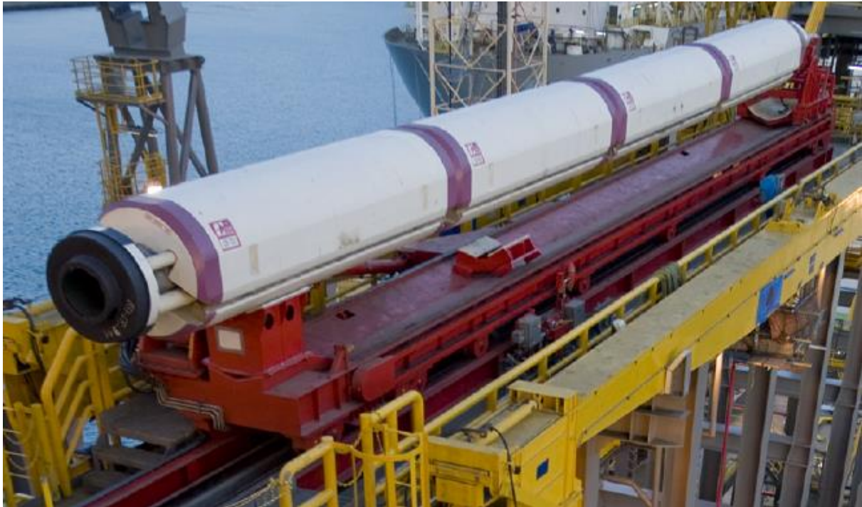
Figure 6: An example of riser joint positioned between the bucket and the riser support supported on the skate located on the rail assembly
