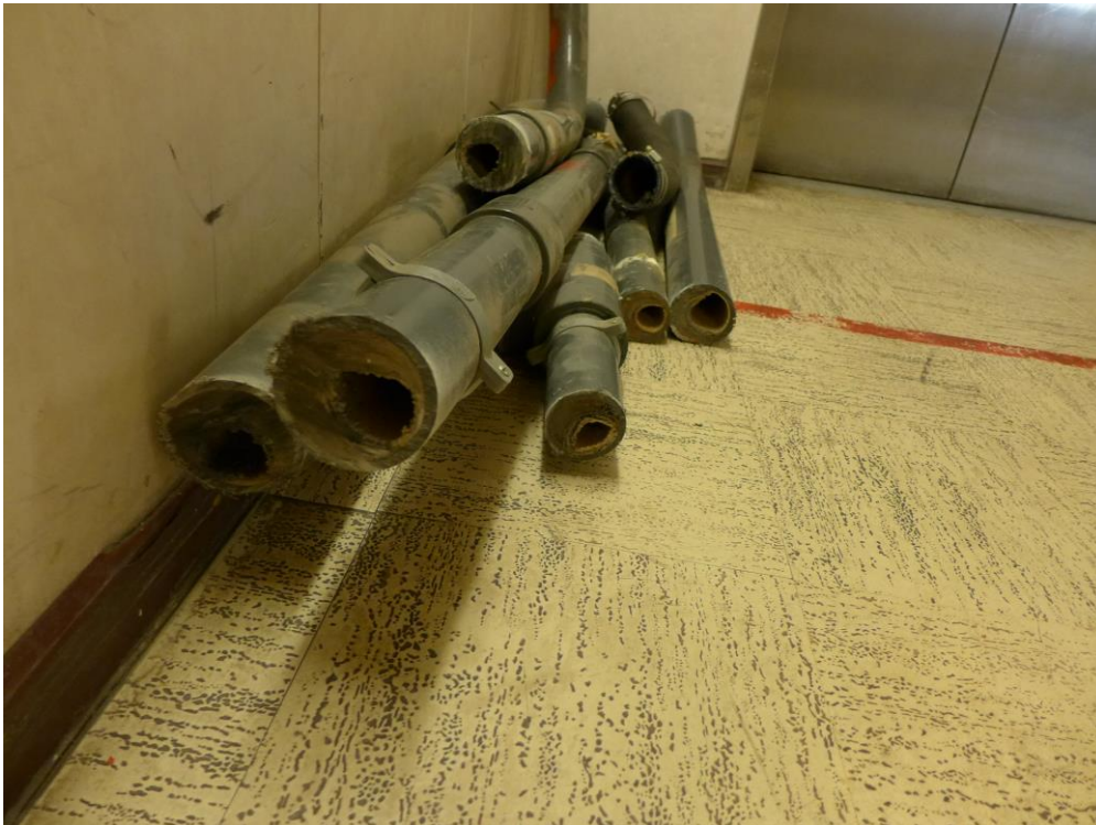
Figure 5: Pipe sections removed due to internal build-up of sediments
