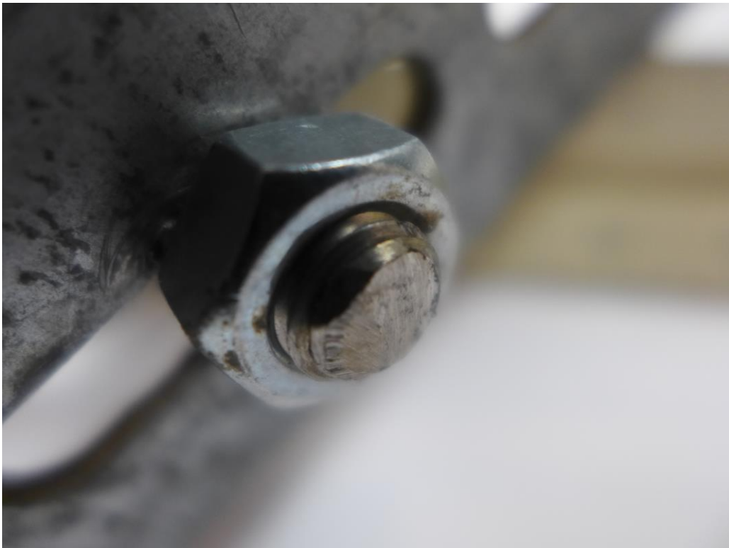
Figure 14: Image of the shortened bolt
