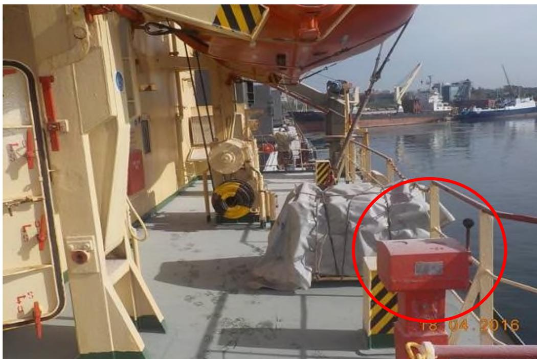
Figure 5: Master controller with hoist speed selection lever (circled)
