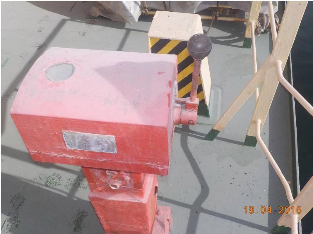
Figure 15: Master controller with two step speed change lever
