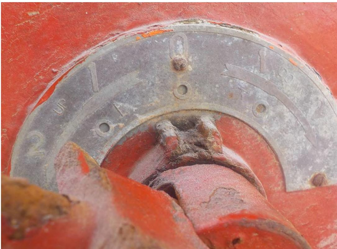
Figure 16: Speed change lever speed control and neutral location
