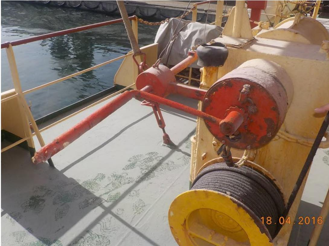
**Figure 13: Winch assembly unit and manual crank-handle**
