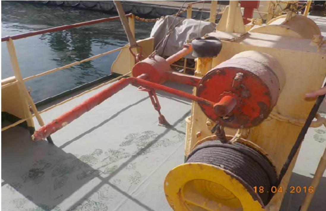
**Figure 10: Winch motor and manual crank-handle devoid of warning notices, operating procedures and hazard identification**
