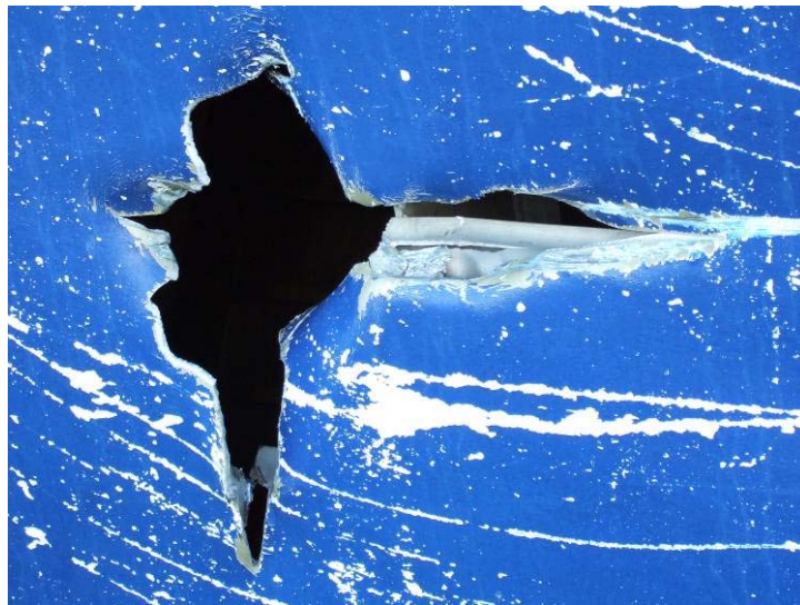
Left: HD1 initial penetration and exit gouge in an astern direction.
