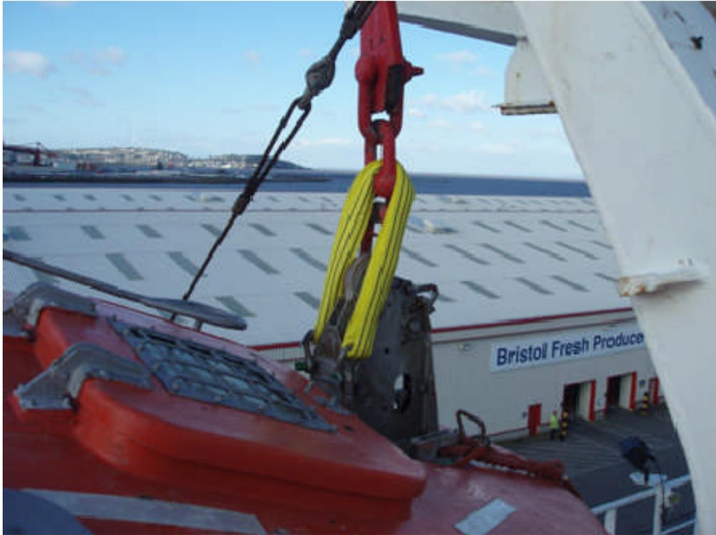
Figure 1 – Continuous sling in place over-riding on-load release
