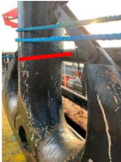
Figure 2: Close up of auxiliary block with the intended position of rope indicated with the red line
