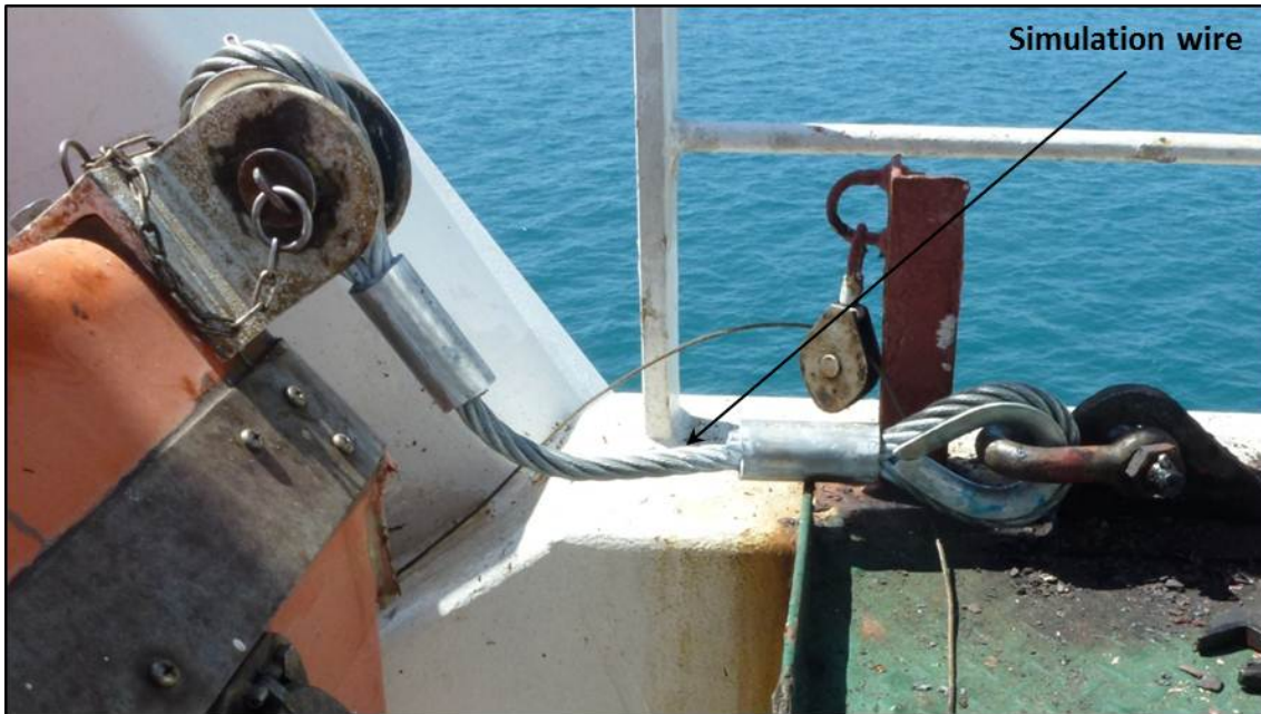
Figure 6: Aft lashing arrangement showing one of the two simulation wires
