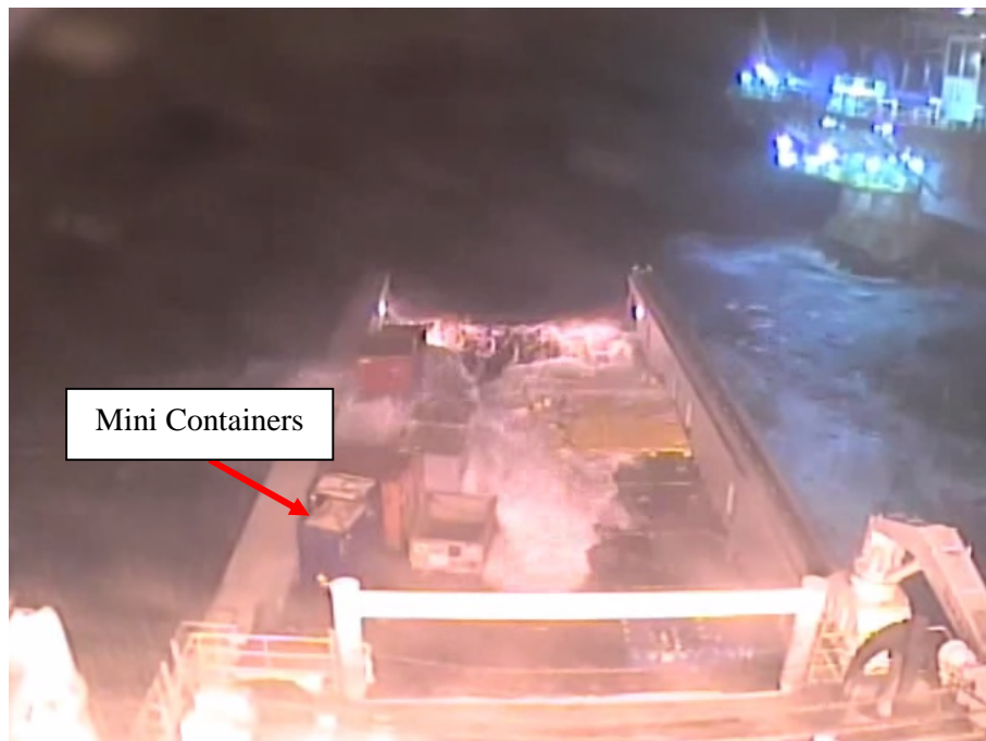
Figure 10: CCTV image of containers moved due to the water force
