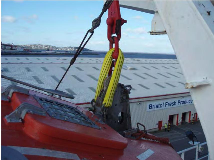
Continuous sling in place over-riding on-load release
