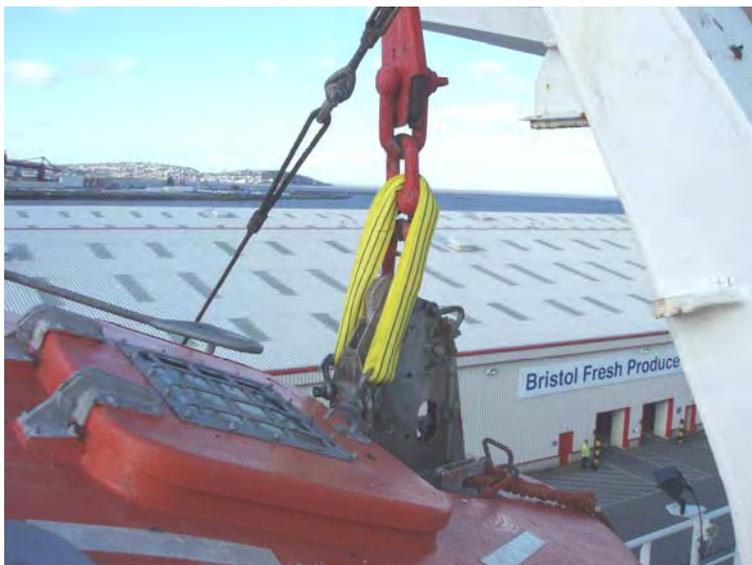
Note: Slings are more suitable as FPDs than are Stropps as they do not have eye splices. This eliminates additional points of weakness. It also enables a shorter connection where this may be necessary.
